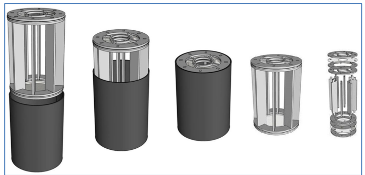
All-in-One Mosquito Containers developed under the CRP on Mosquito Handling, Transport, Release and Male Trapping Methods.
