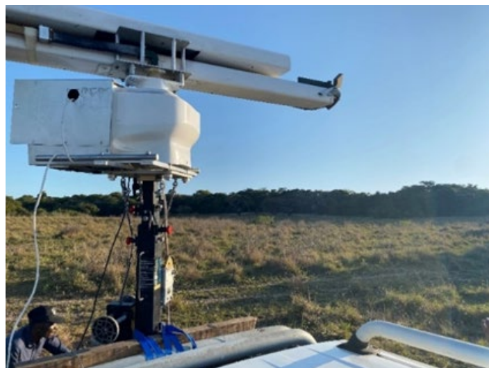
Radar setup operated in the field test in Mozambique to detect tagged Glossina brevipalpis .
