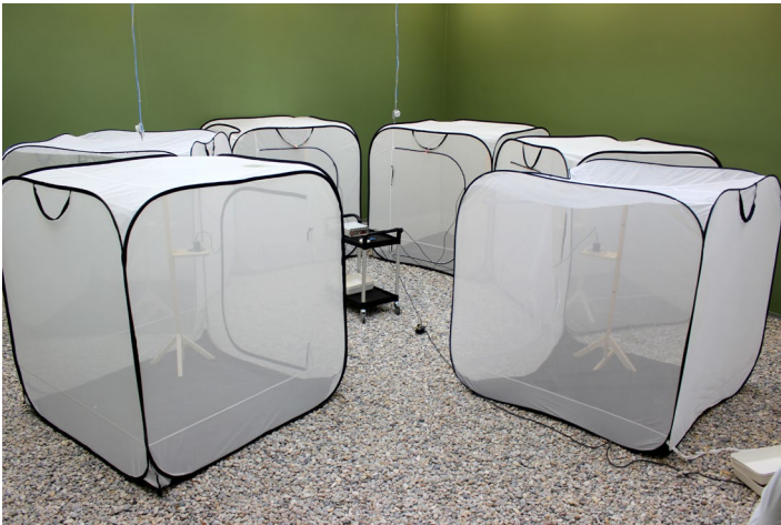
Irradiated sterile, and non-irradiated fertile male mosquitoes competing for virgin mature non-sterile females in semi-field cages to evaluate the mating competitiveness of sterile males following various treatments.
