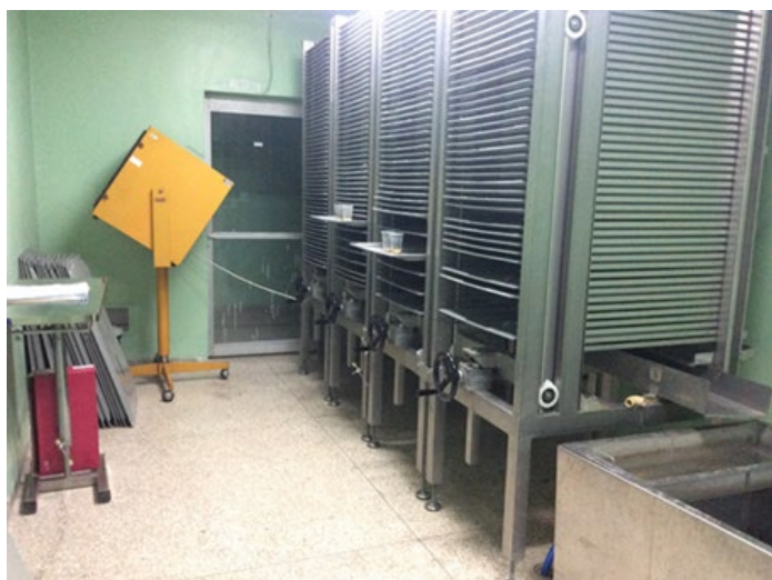
Equipment for the mass-rearing of Aedes aegypti installed at the Institute of Tropical Medicine ‘Pedro Kouri’ (Photo: Rene Gato).
