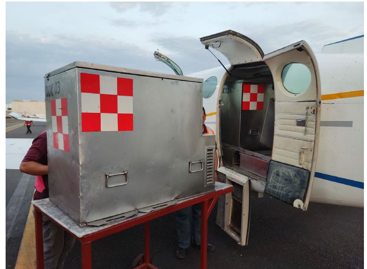
A release box containing some 15 million sterile male Mediterranean fruit flies being loaded to a Cessna aircraft for release over Colima, Mexico. (Photo: DGSV Senasica).
