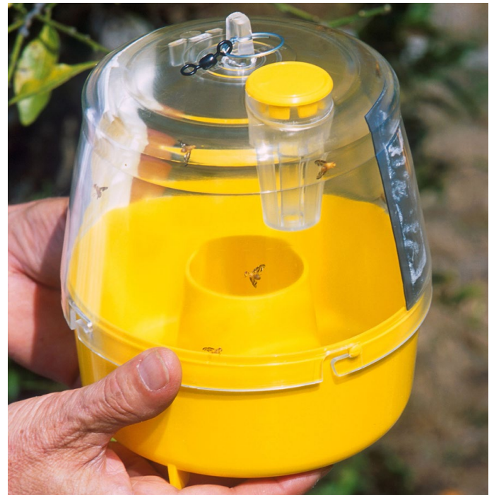
Multilure trap used for a wide range of attractants and fruit fly species (Photo: IAEA).
