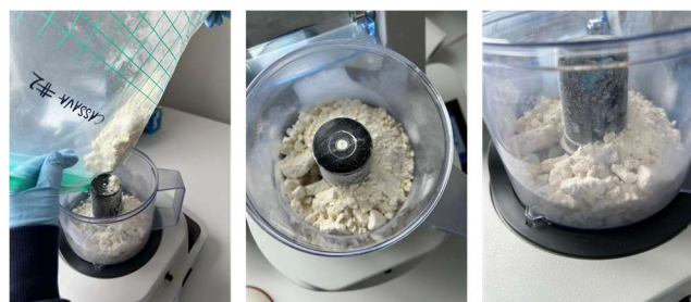
Figure 2: Second processing of the freeze-dried cassava roots in a sample homogenizer (Photo courtesy of Ms B. Maestroni)
