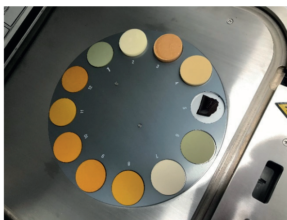
FIG. 2. Turmeric samples are analysed together with NIST reference materials in the ED-XRF.
