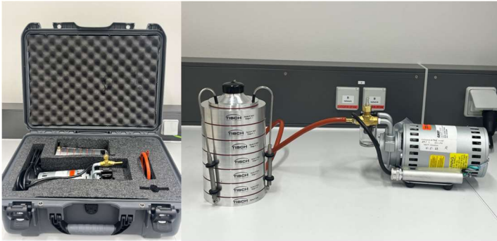
Impactor bioaerosol samplers for detection and characterization of AMR in animal farms
