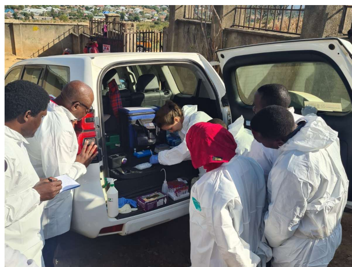
Bringing ASF Diagnosis to the Front Lines: On-site Nucleic Acid Extraction and real time PCR Amplification of ASFV at an Iringa Abattoir, Tanzania
