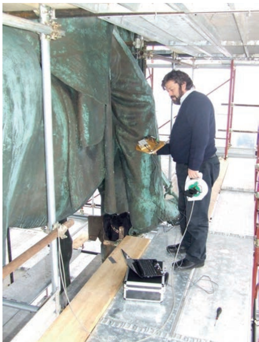
Fig 1. XRF technique applied for characterization of the Garibaldi statue in Rome.
