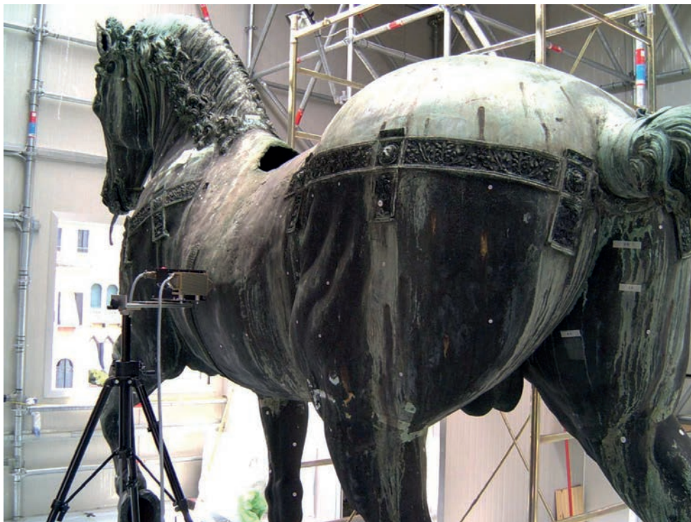
Fig.5. XRF measurements on the horse of the Colleoni statue in Venice.
