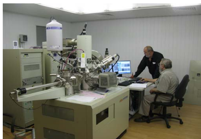
Fig.4. The advanced instrument which combines: field-emission gun SEM/EDX, micro-XRF with capillary optics and Auger electron spectrometry with an argon-ion gun.
