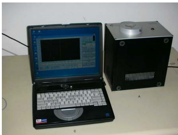
Fig. 1. X ray tube-based portable XRF analyser
