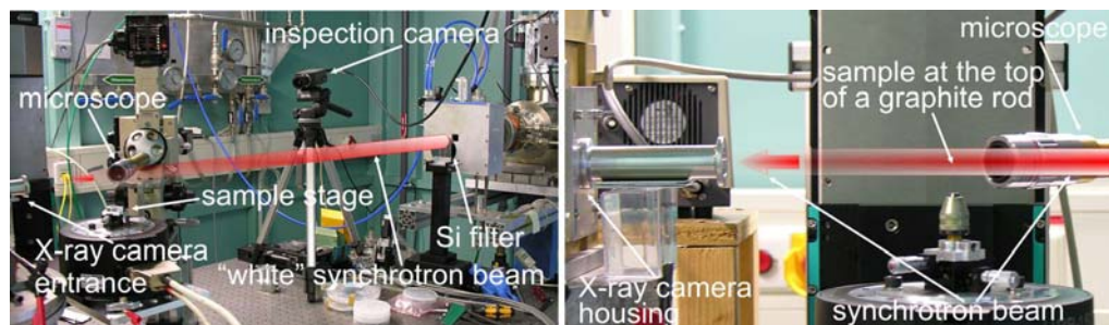
Fig. 1. X ray phase contrast imaging set up at the TOPO beamline, ANKA Synchrotron Facility. Left picture shows overall view of the set up, in the right-hand side picture a close up view of the "sample - X ray camera" region is shown.
