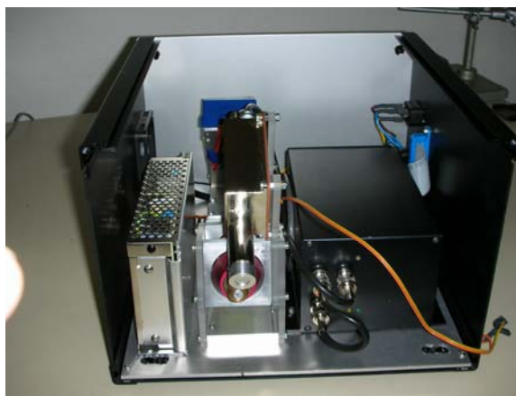
Fig. 1. X ray tube-based portable XRF analyser
