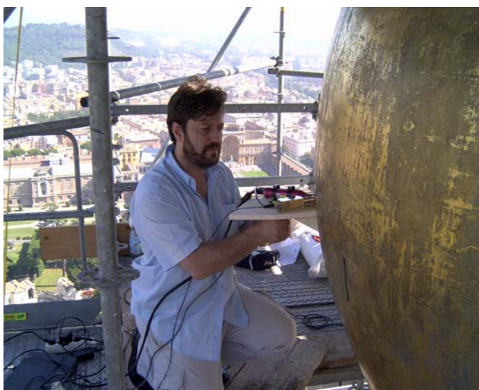
Fig. 2. Outside XRF measurements on top of the Cupola of Saint Peters' Basilica in Rome
