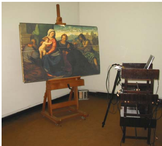
Fig. 1. The XRF system in front of the analysed painting in Belgrade
