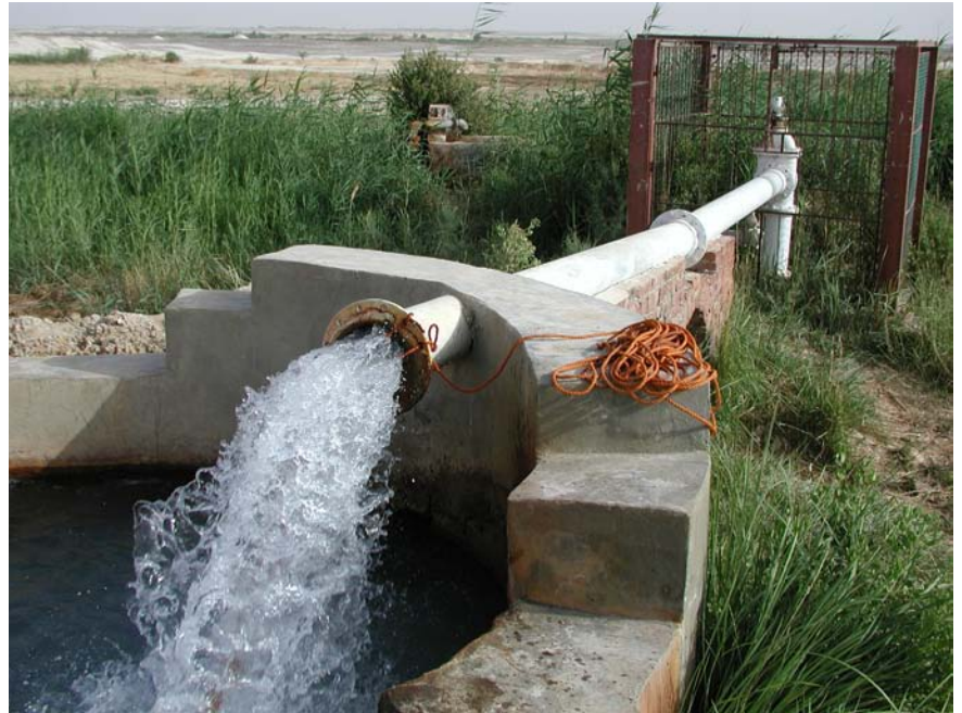
Nubian Aquifer water being sampled from well #6 at Farafra Oasis, Egypt, for ^{81}\text{Kr} analysis. A plastic tube was inserted into the discharge pipe to minimize the risk of air contamination during sampling (Photo credit: Zheng-Tian Lu).
