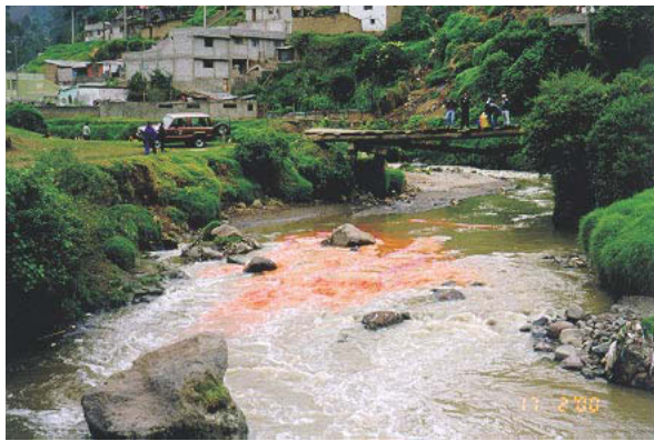
Injection of the cocktail of tracers in the Machangara and Guayllabamba rivers
