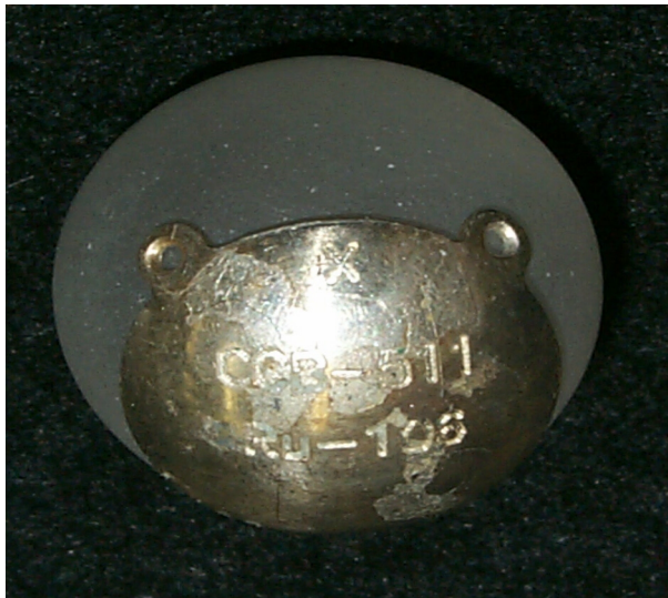
FIGURE 3. ^{106}\text{Ru}/^{106}\text{Rh} ophthalmic applicator with two suture holes.
