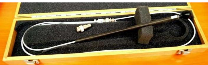
Figure 1. Exradin A3 chamber
