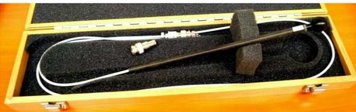
Figure 1. Exradin A3 chamber
