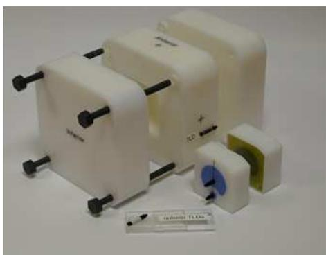
*Fig. 2. Solid phantom for ‘end-to-end’ dosimetric quality audit for IMRT including imaging, treatment planning and delivery.*
