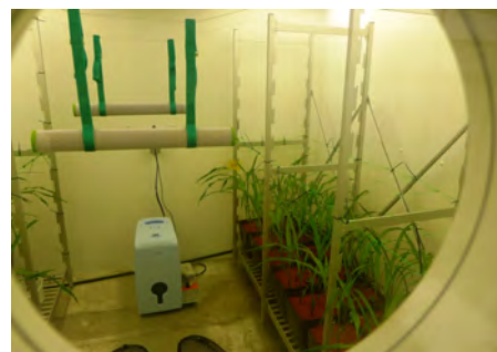
Figure 2. Carbon-13 labelling of maize in ^{13}\text{C}\text{-CO}_2 analyser controlled walk-in growth chamber at the SWMCNL Laboratory
