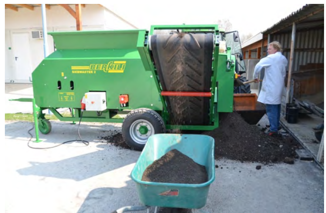
Fig. 1. Motor operated rotary drum soil sieve machine increases the efficiency of preparing soils for pot and cosmos experiments.
