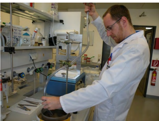
Fig. 1: Using the low-cost micro-aggregate isolator to extract soil fractions according to Six et al., 2002.
