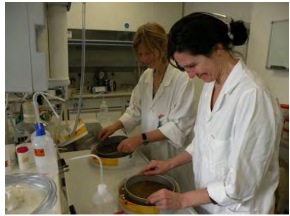
Fig. 2: Wet sieving of soil for separating soil fractions.
