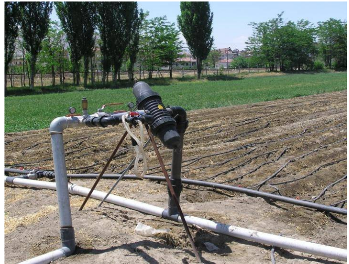
Drip irrigation-fertigation system at Niğde Potato Research Institute for the Demonstration Experiment where potato crop was just planted
