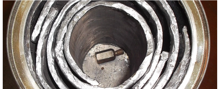
In the absence of an appropriate lead container, the source was placed in an “internal container” that was engineered with available materials and with layers of lead. (Photo: IAEA)
