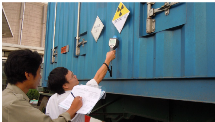
Experts ensure there is adequate shielding of the radioactive material.
