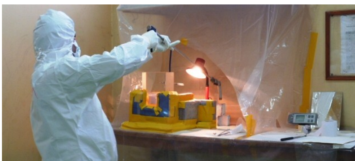
Egyptian operator takes the source out of its container to condition it for safe disposal. (Photo: IAEA)
