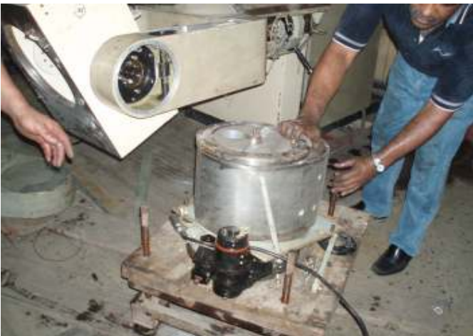
Dismantled Russian teletherapy head
