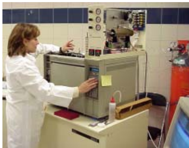
The GC-C-IRMS instrument to measure the stable carbon isotope ratios ( \delta^{13}\text{C} ) of individual organic compounds.
