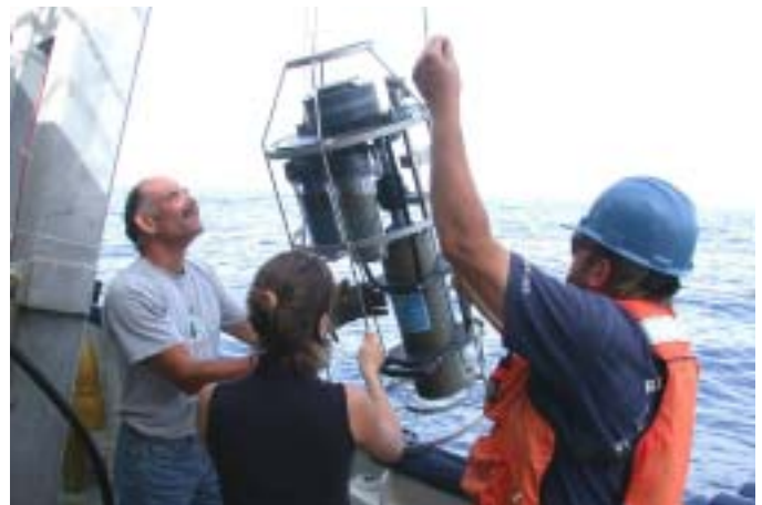
Field sampling large volume in-situ pump to collect particulate material and the dissolved phase of specific elements.
