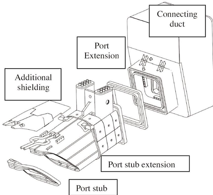
Fig. 2. Exploded view of upper port structure
