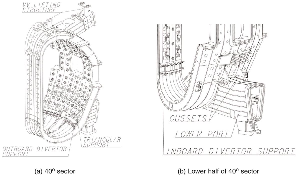
Fig. 1. The ITER Vacuum Vessel
