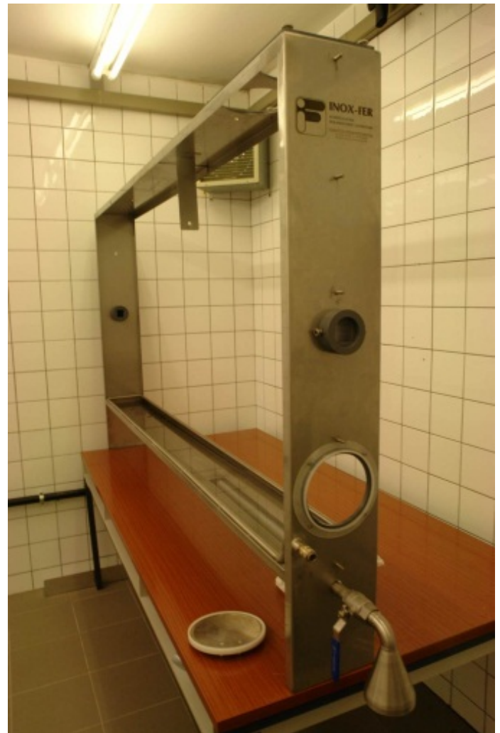
Prototype of mass-rearing cage for Anopheles arabiensis .
