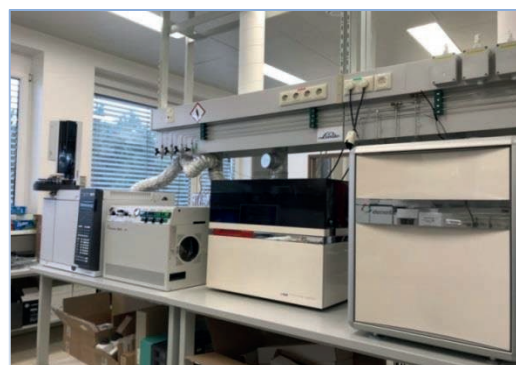
The new Elementar VisION system. From left to right; the Agilent 7890B Gas Chromatograph ; The GC5 combustion and pyrolysis interface; the VisION gas isotope ratio mass spectrometer and the PyroCube elemental analyser.
