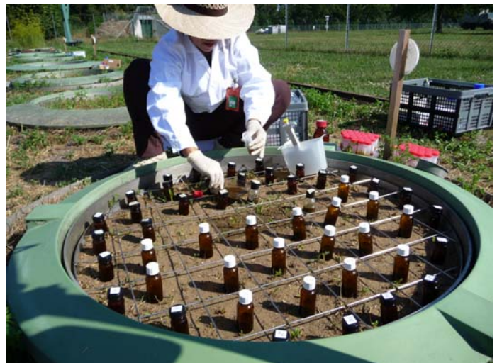
Lysimeter facilities showing the application/sampling grid
