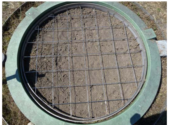
Lysimeter facilities showing the application/sampling grid
