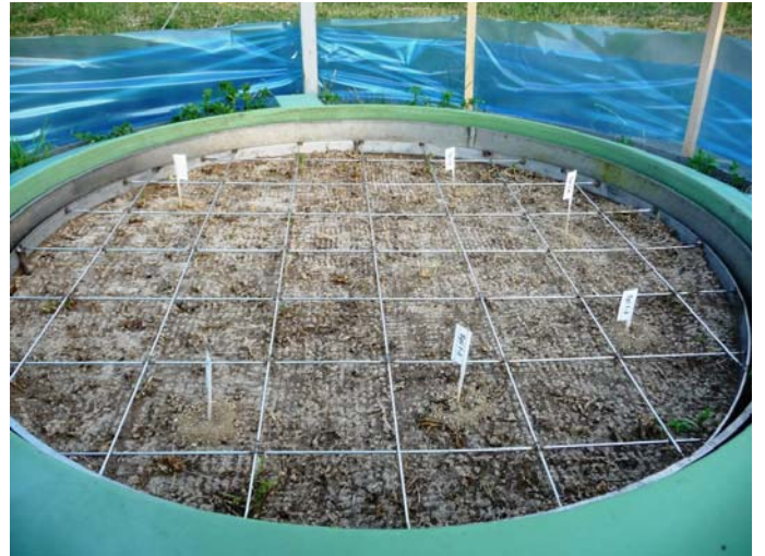
Application of slurry containing 14 C-labeled levamisole and other anthelmintics
