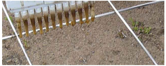
Application of slurry containing 14 C-labeled levamisole and other anthelmintics
