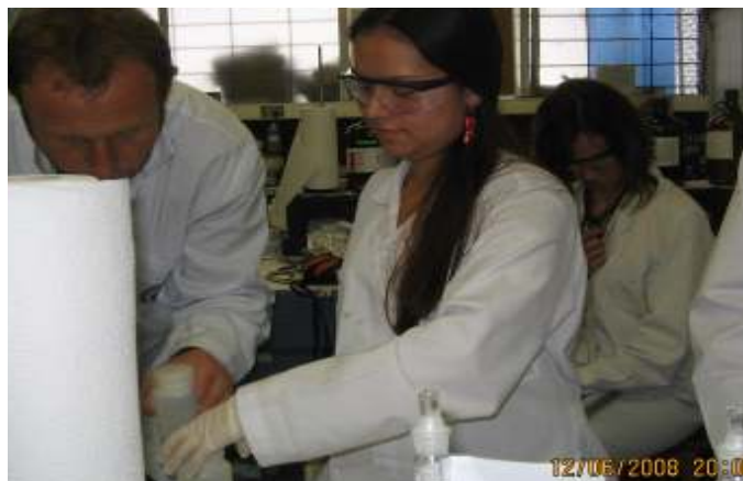
Ms. Jessie Materita and Dr. Berthold Kettner conditioning SPE columns for the clean-up step for analysis of pesticides in water
