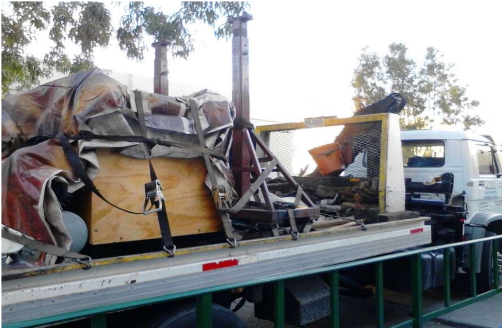
FIG. 3. Transport of the teletherapy unit head with the ^{60}\text{Co} source to the waste disposal facility (picture captured prior to the incident) (courtesy of CNSNS).
