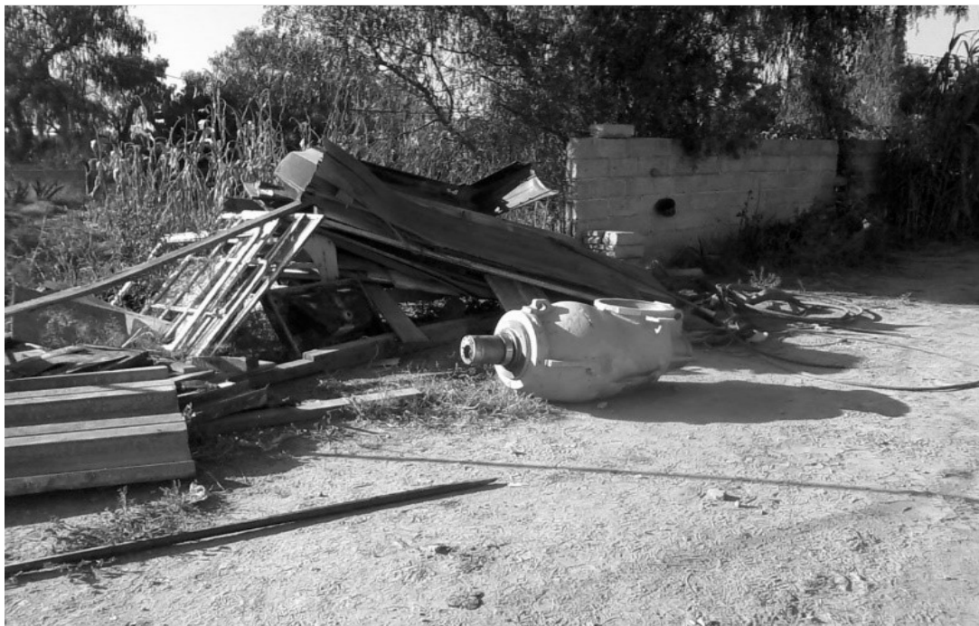
FIG. 5. The empty radioactive source shielding (courtesy of CNSNS).
