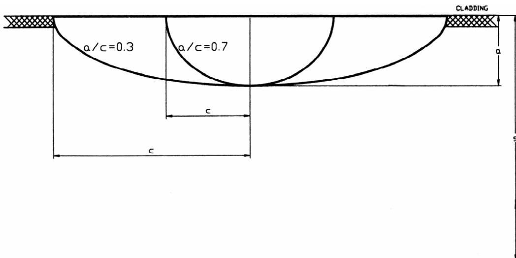
FIG. 5 Semielliptical surface crack, cladded vessel.
