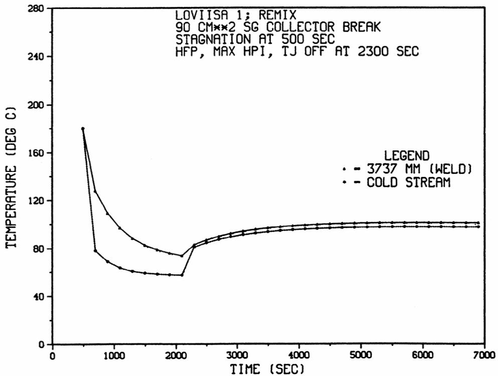
FIG. 11. REMIX calculation for sequence "Steam generator collector break ( $90\text{ cm}^2$ ) starting from hot full power conditions". TJ is high pressure injection.
