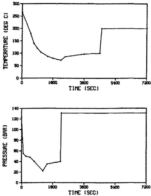
FIG. 12. Downcomer temperature and primary pressure for sequence "Steam generator collector break (90 cm<sup>2</sup>) starting from hot full power conditions", 15 x 50 mm surface crack.  $T_k = 135^\circ\text{C}$ .
