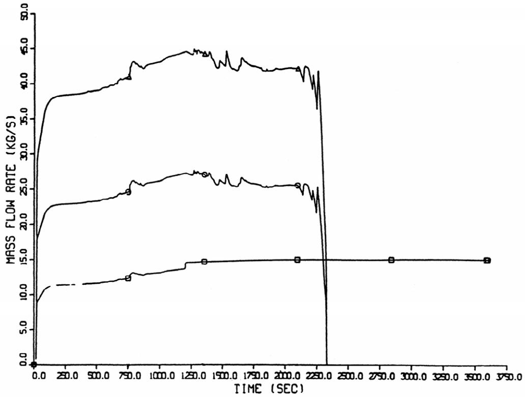
FIG. 10. HPI flow rates into the single ( $\square$ ), double ( $\circ$ ) and triple ( $\Delta$ ) loop in RELA P5/MOD2 calculation for sequence "Steam generator collector break ( $90\text{ cm}^2$ ) starting from hot full power conditions".
