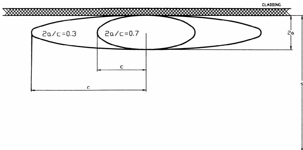
FIG. 3. Elliptical undercladding crack, cladded vessel.
