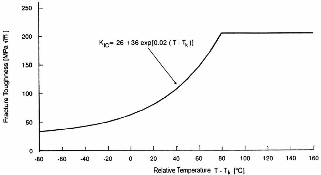
FIG. 6. Allowable stress intensity factors for WWER RPV steels.
