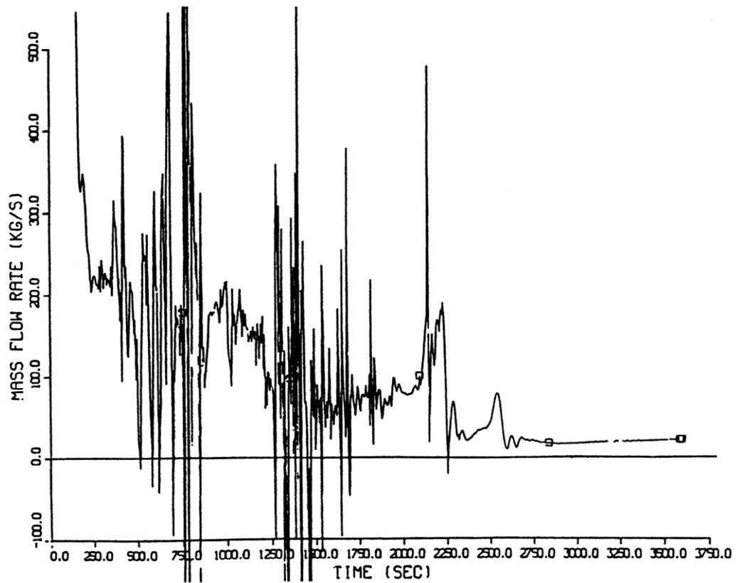
FIG. 8. Mass flow rate in the downcomer in RELA P5/MOD2 calculation for sequence "Steam generator collector break (90 cm<sup>2</sup>) starting from hot full power conditions".
