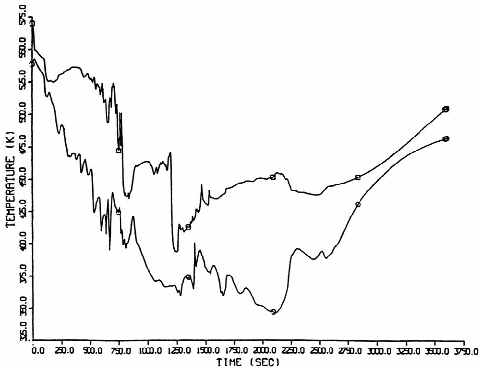
FIG. 9. Hot leg (□) and downcomer fluid temperature (○) in RELA P5/MOD2 calculation for sequence "Steam generator collector break (90 cm<sup>2</sup>) starting from hot full power conditions".
