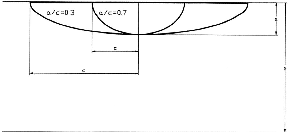
FIG. 2. Semielliptical surface crack, uncladded vessel.
