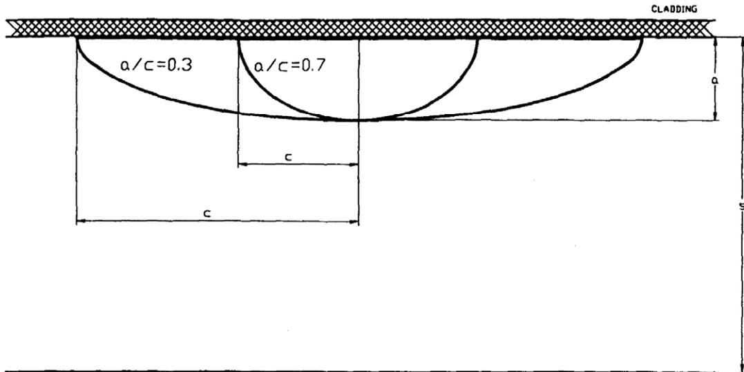
FIG. 4 Semielliptical undercladding crack, cladded vessel.
