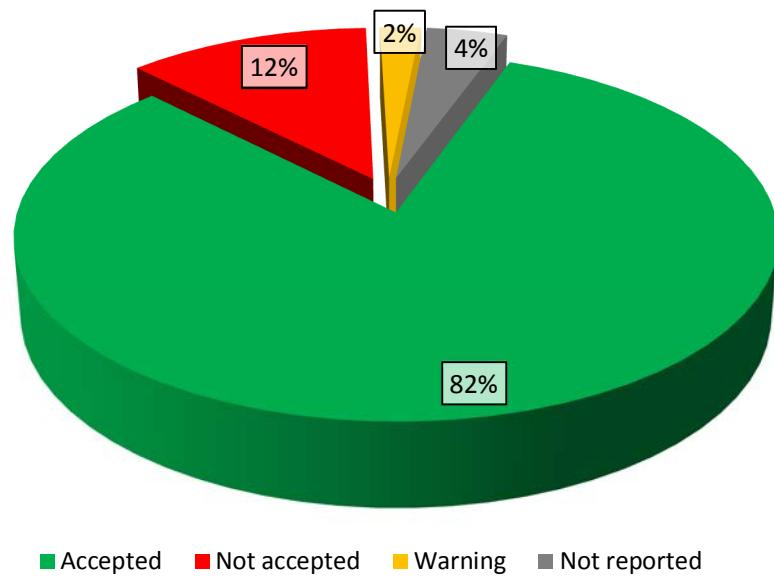
*FIG. 37. Distribution of the scores for Ba-133 in water (sample 02).*
