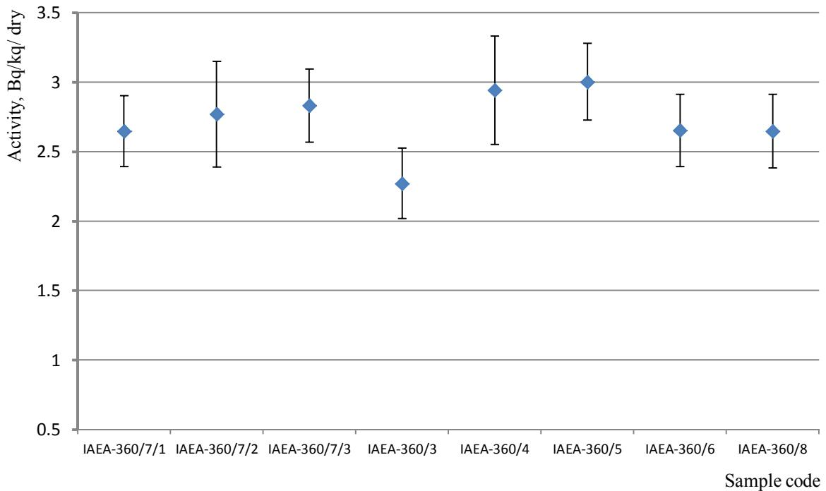
*FIG. 5. Results of the determination of Sr-90 (activity calculated for the reference date October 2009).*
