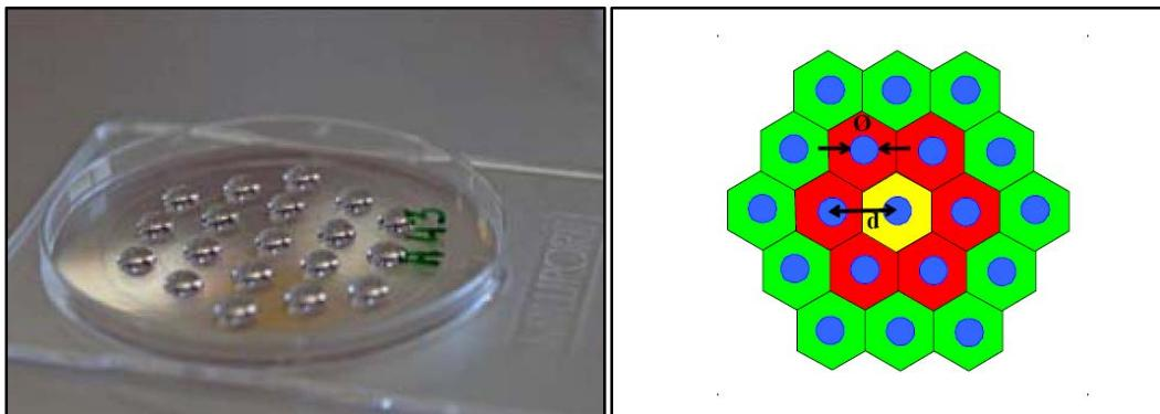
*FIG. 3. The pattern of the simulated aerosol filter.*
