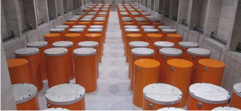
FIG. 23. Dry storage in CONSTOR concrete casks NPP Ignalina, Lithuania (courtesy of State Enterprise Ignalina Nuclear Power Plant).
