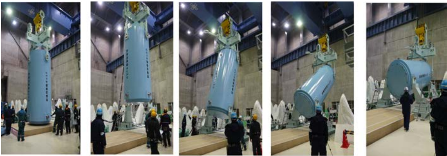
FIG. 57. Cask handling training using a mock-up cask (Copyright: RFS 2019. Unauthorized use or reproduction of this image is prohibited).
