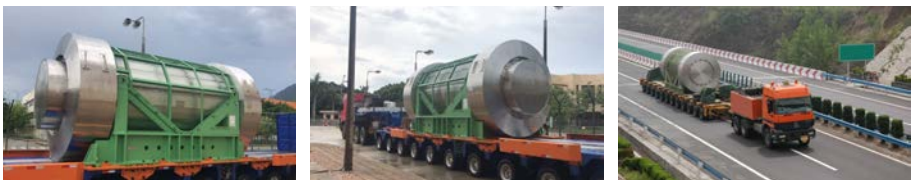
FIG. 52. NAC-STC transport cask being transported by truck on road (courtesy of NAC).
