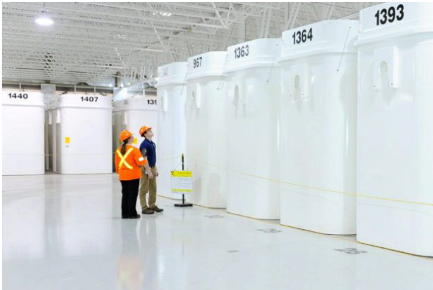
FIG. 22. Ontario Power Generation's concrete dry storage container; Canada.
