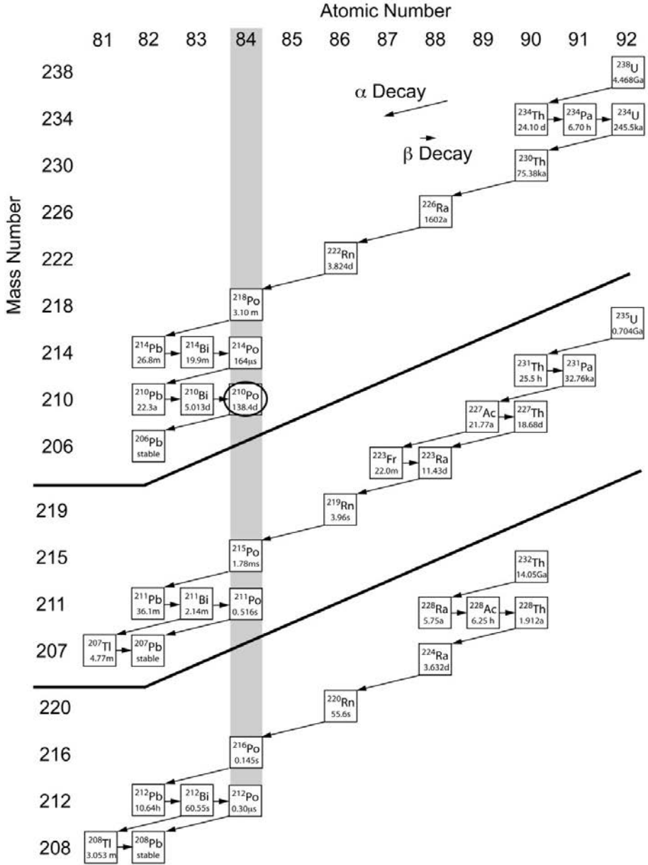
FIG. 3.1. The naturally occurring ^{238}\text{U} , ^{235}\text{U} and ^{232}\text{Th} decay series, all of which contain polonium isotopes ( Z = 84 ).
