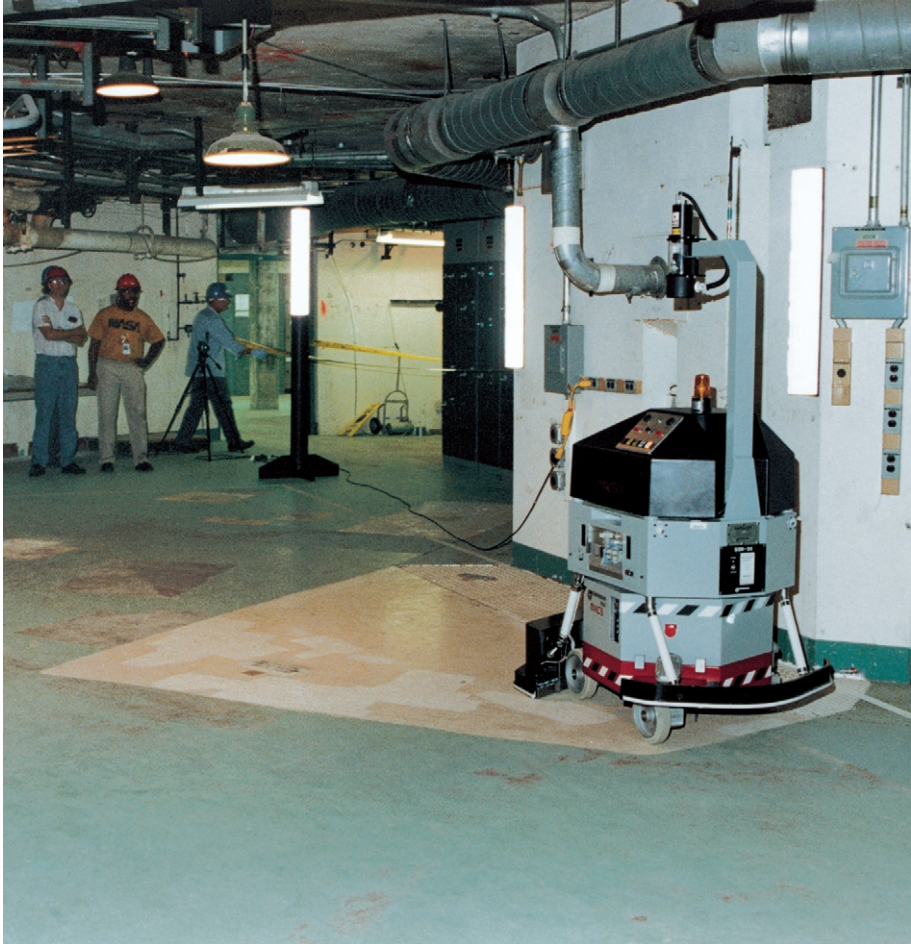
FIG. 46. The mobile automated characterization system robot being used for floor radiation surveys at the CP-5 facility.
