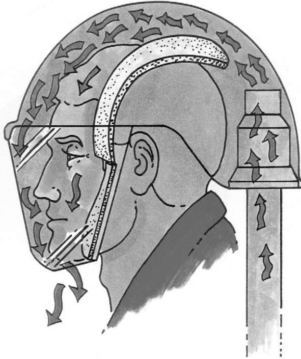
FIG. 50. Protection helmet to prevent the inhalation of radioactivity. Clean pressurized air is fed into the back of the helmet and passes over the wearer's head, thereby preventing the inhalation of loose radioactive particulate. An additional advantage is that the air flow prevents condensation forming within the helmet.
