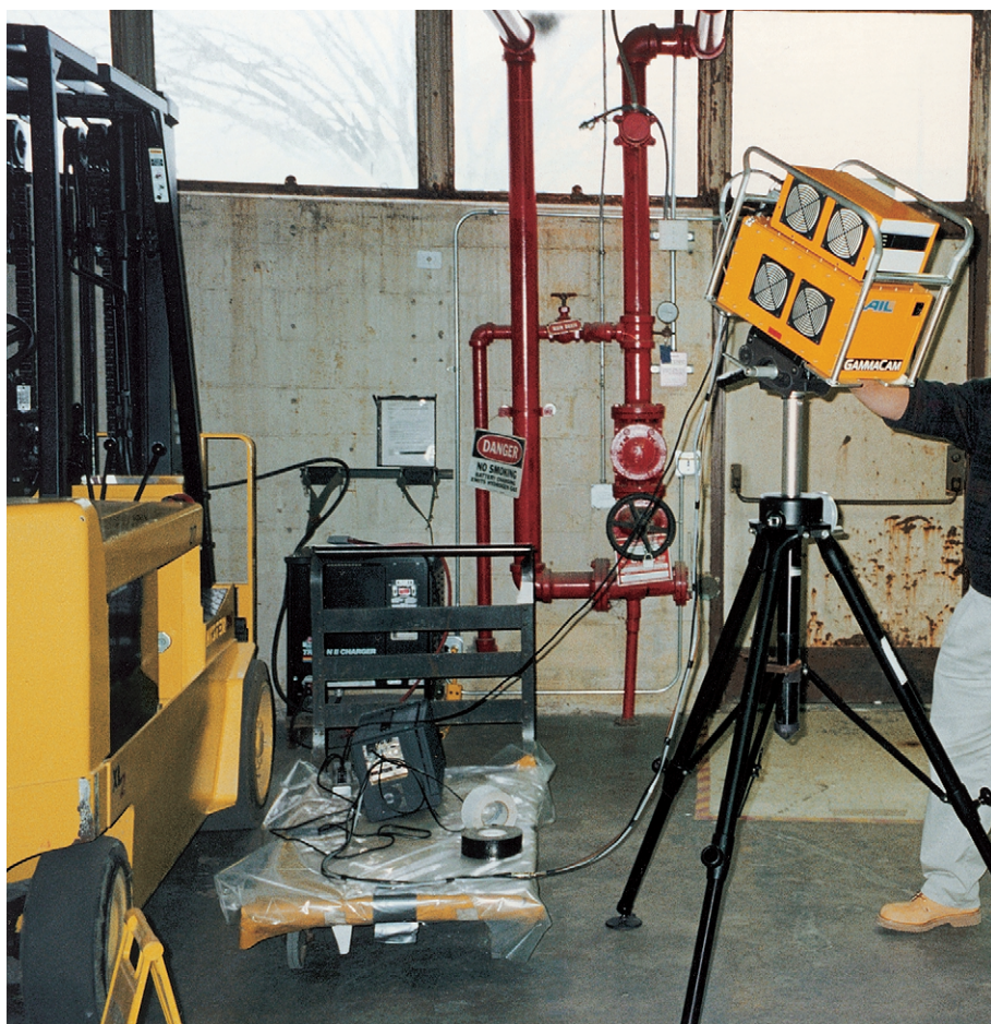
FIG. 47. Gamma camera as used for gamma radiation field imaging at the CP-5 facility.
