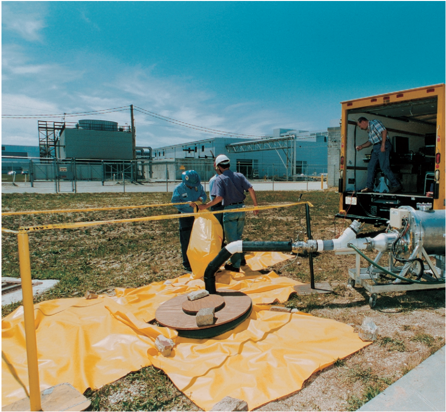
FIG. 45. Pipe Explorer™ being used to perform characterization of the CP-5 facility's embedded piping system. Courtesy Argonne National Laboratory, managed and operated by the University of Chicago for the US Department of Energy under contract No. W-31-109-ENG-38.
