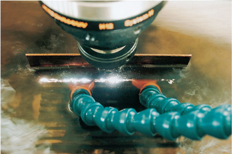
FIG. 36. EDM being tested on cutting thick gauge metal (underwater for remote use) at the BR3 decommissioning project.
