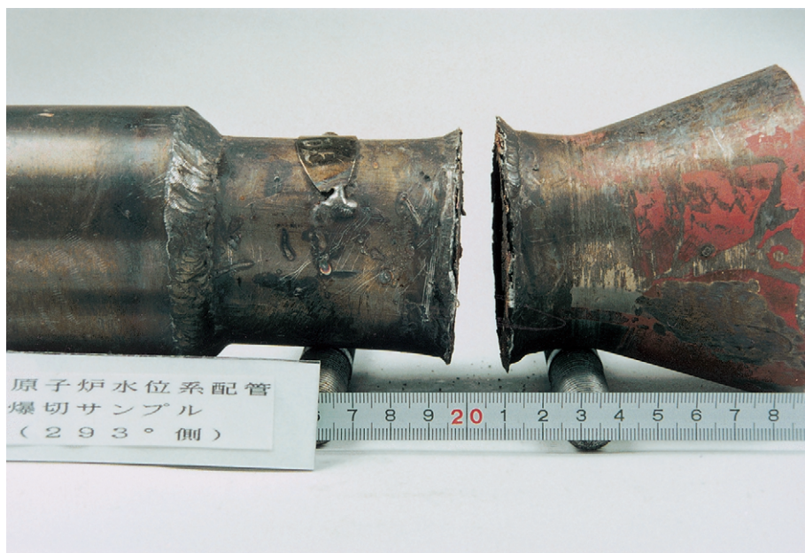
FIG. 27. Emergency condensate system pipe cut by shaped explosive, JPDR decommissioning project.
