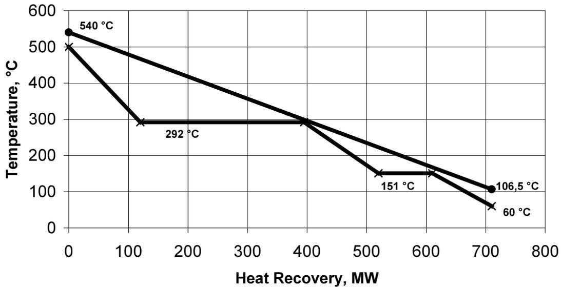
Fig. 6. Temperature/heat recovery diagram of the HRSGs.
