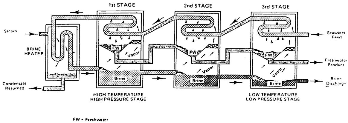
Fig. 2. Schematic flow diagram of an MSF system.
