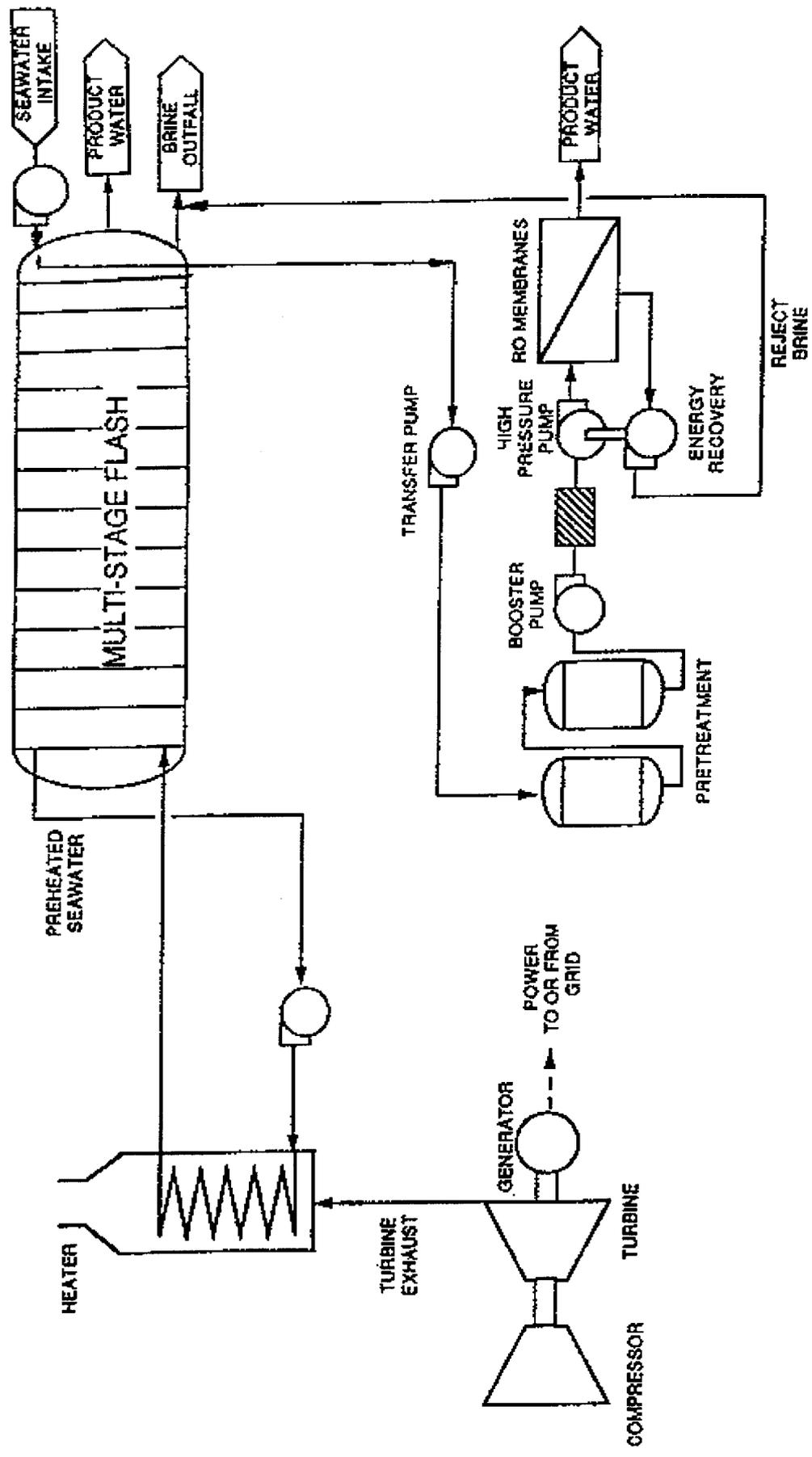
FIG. A-18. Fossil gas turbine with hybrid MSF and RO.
