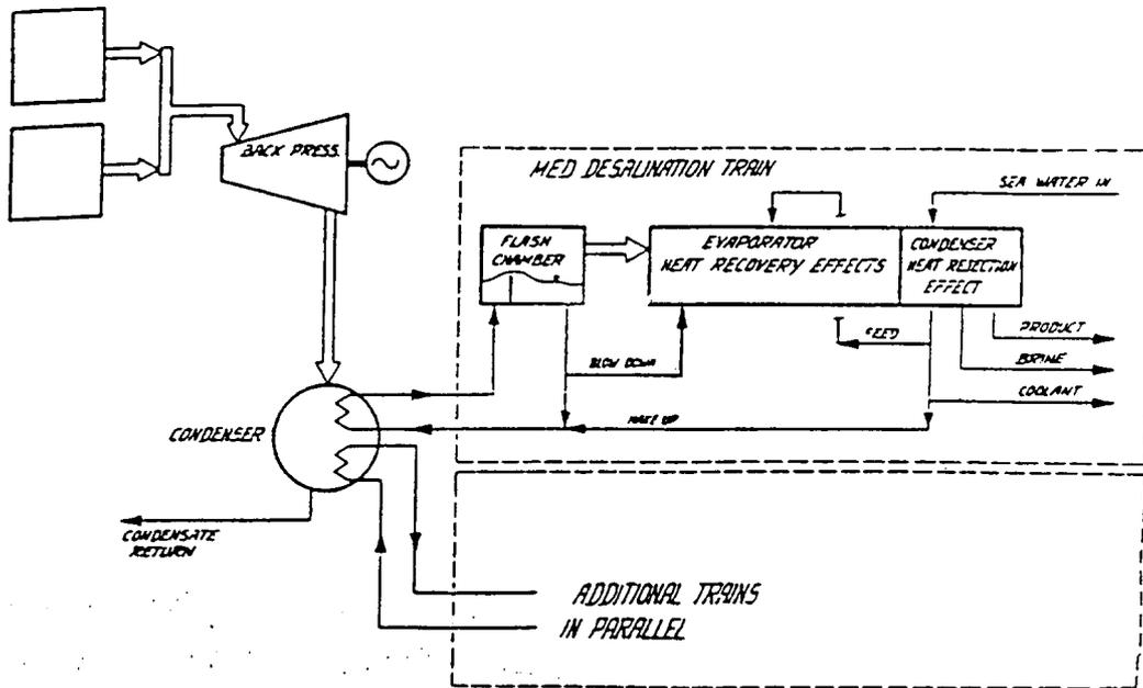
Fig. 10. Flash loop between backpressure condenser and MED units.
