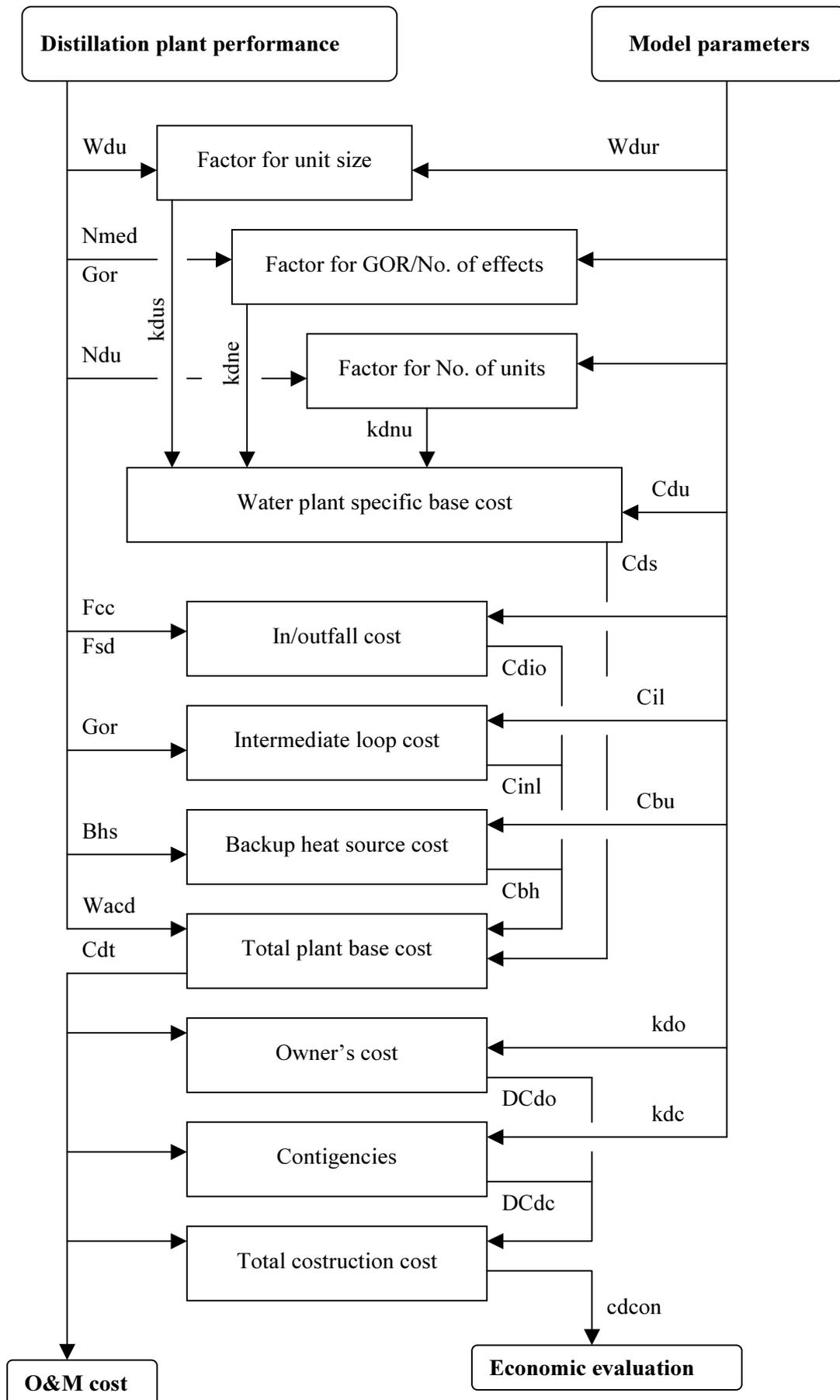
Fig 30. Distillation plant construction cost.
