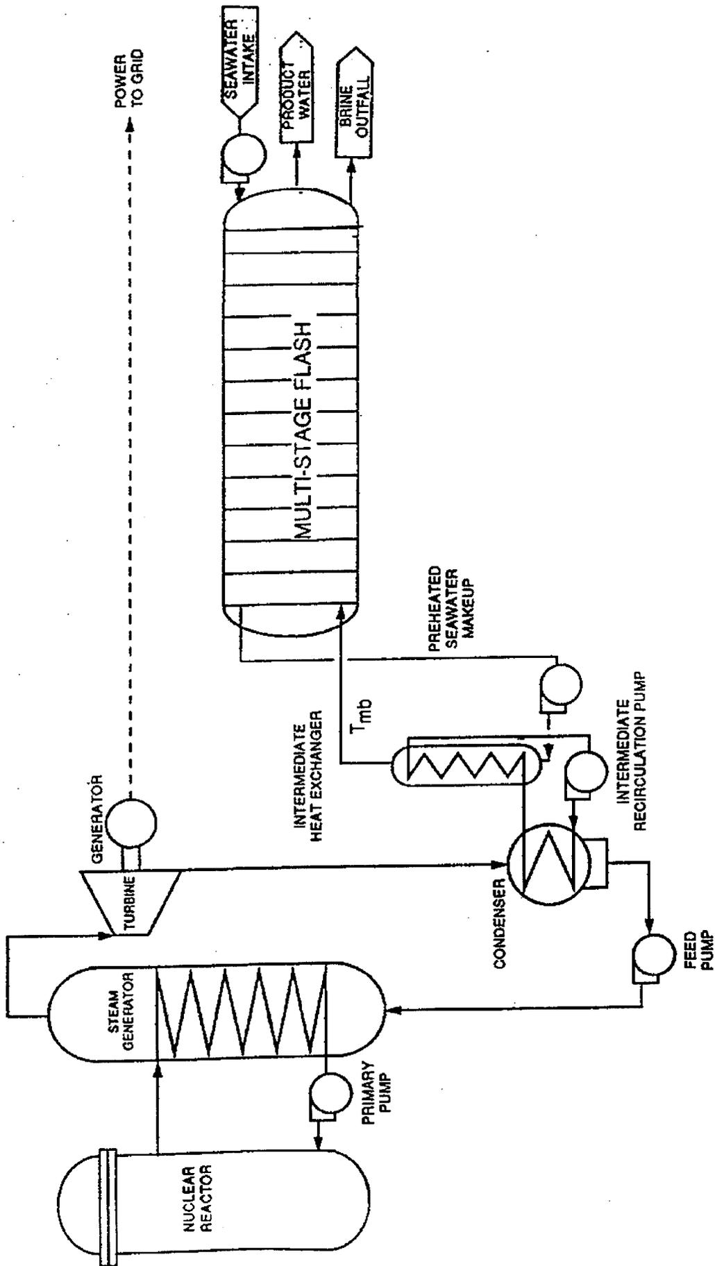
FIG. A-2. Nuclear power reactor with backpressure steam cycle and MSF.
