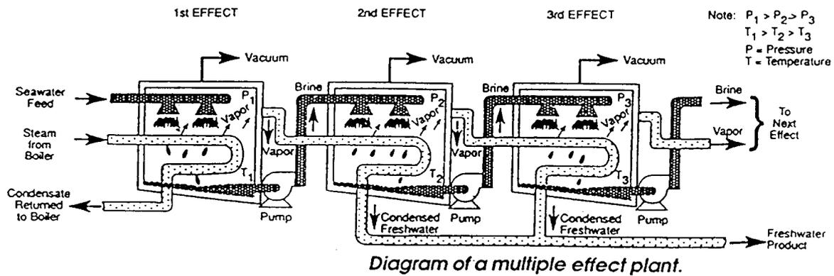
Fig. 3. Schematic flow diagram of an LT-HTME plant.
