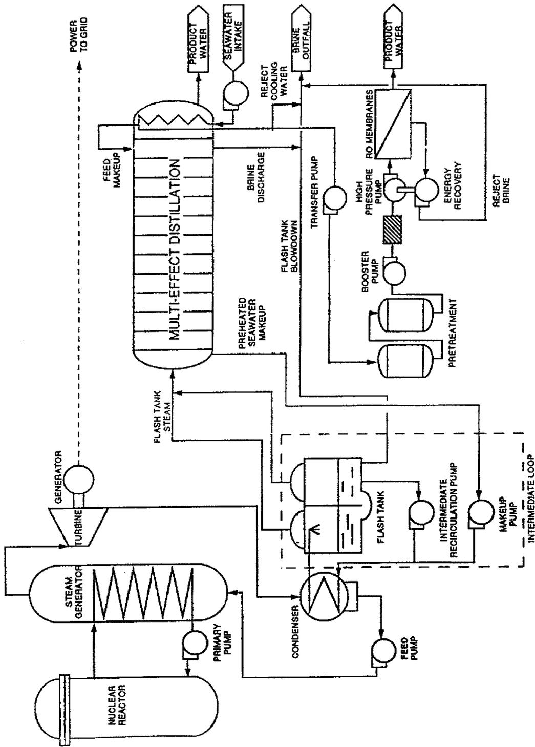
FIG. A-5. Nuclear power reactor with hybrid MED and RO.
