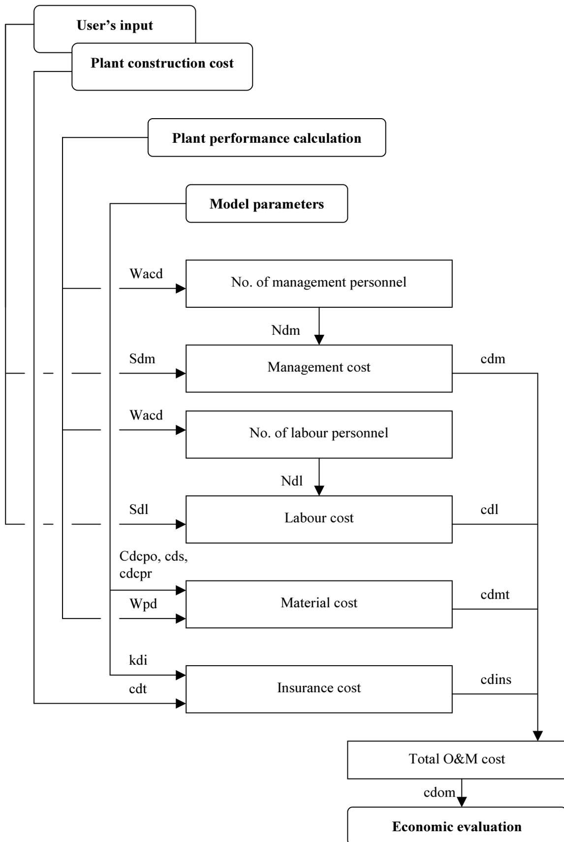
Fig 31. Cost calculation – O&M cost of distillation plant.
