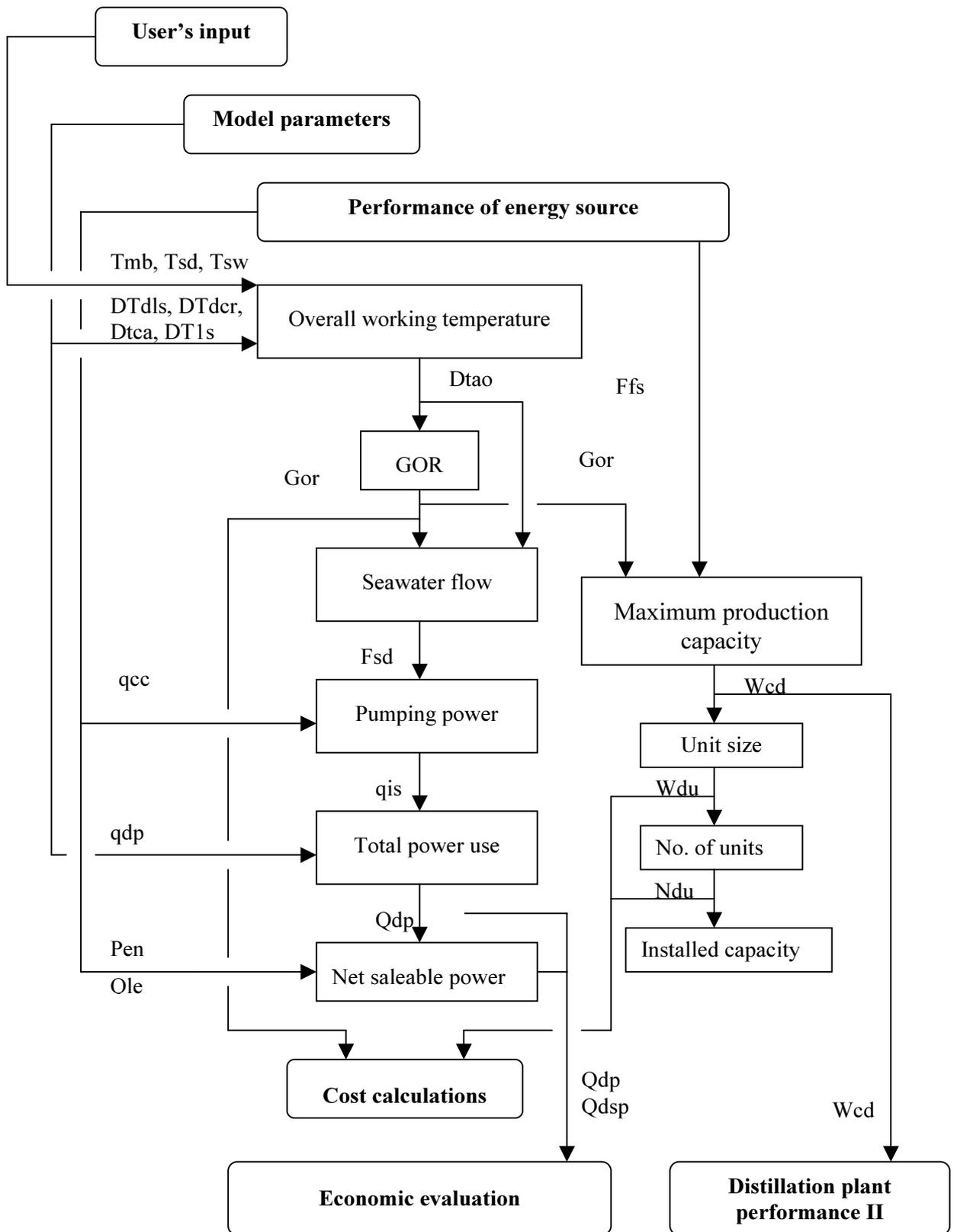
Fig 18. Distillation plant performance I – Calculation of water production capacity.
