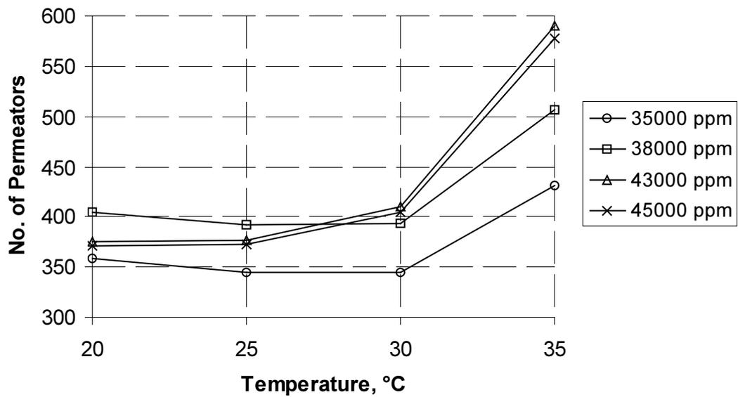
Fig 28. Number of permeators of hollow fibre membranes.
