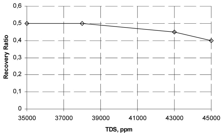
Fig 26. Recovery ratio of hollow fibre membranes.
