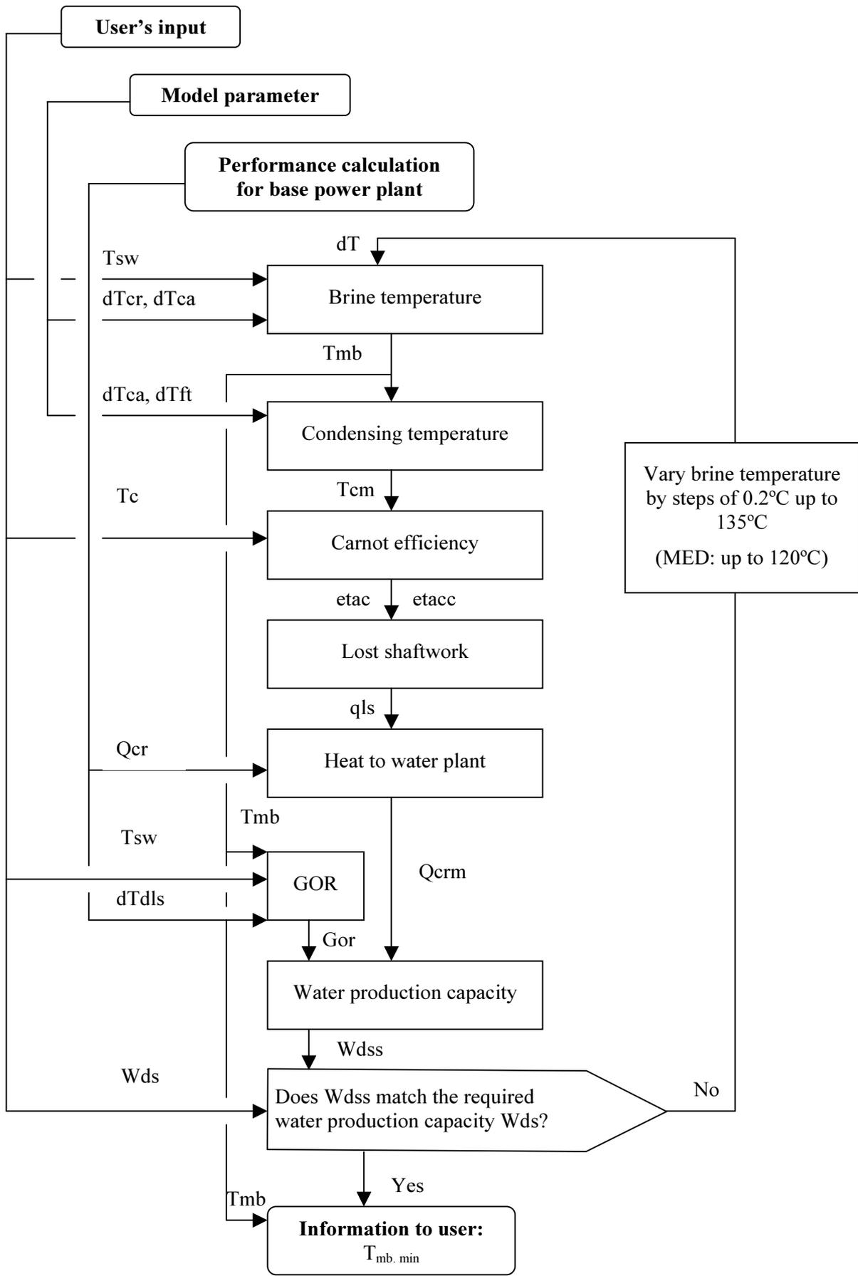
Fig 17. Calculation of the minimum required maximum brine temperature for a MSF plant.
