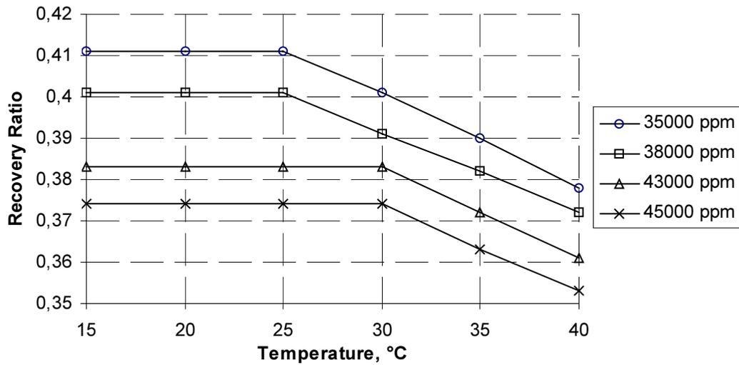
Fig 23. Recovery ratio of spiral wound membranes.
