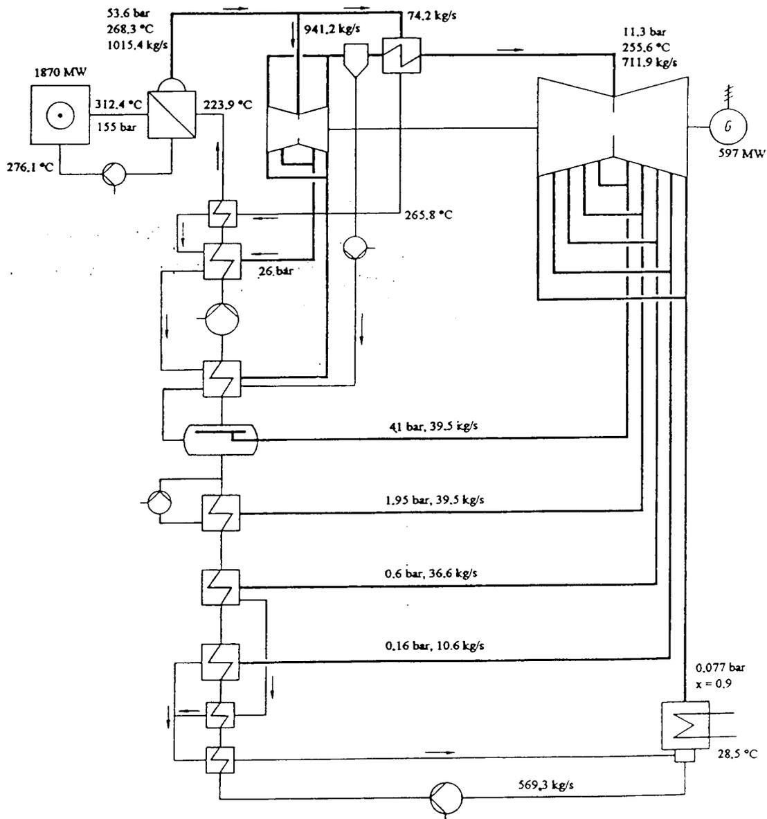
Fig. 4. Schematic flow diagram of the reference PWR power plant.
