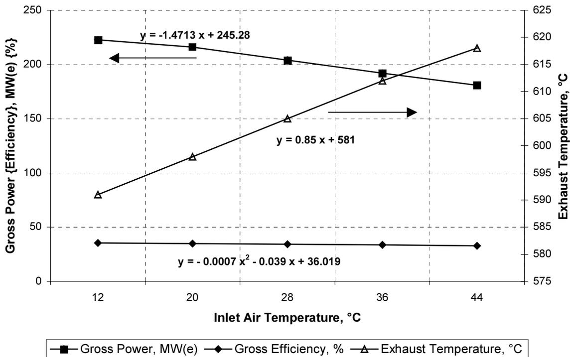
Fig 14. Performance characteristics of the advanced GT plant.
