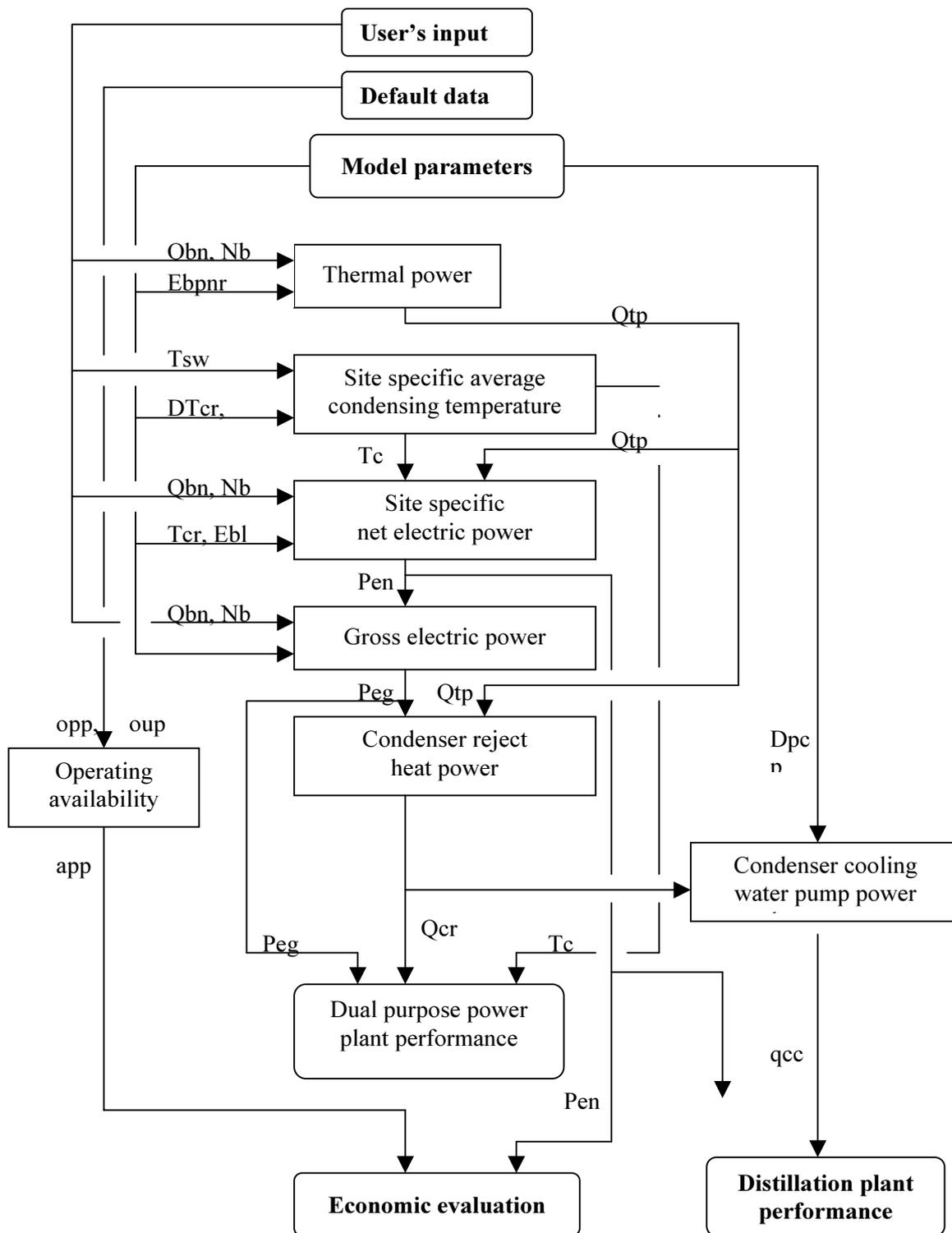
Fig 12. Performance calculation for base steam power plant.
