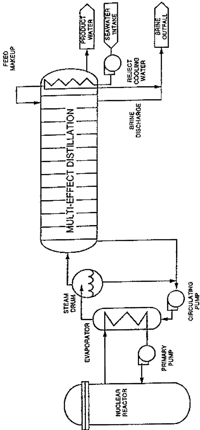
FIG. A-26. Nuclear heat reactor with MED.
