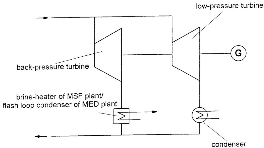
Fig. 8. Coupling of the distillation plant with the PWR power plant (backpressure turbine and low pressure condensing turbine in parallel).
