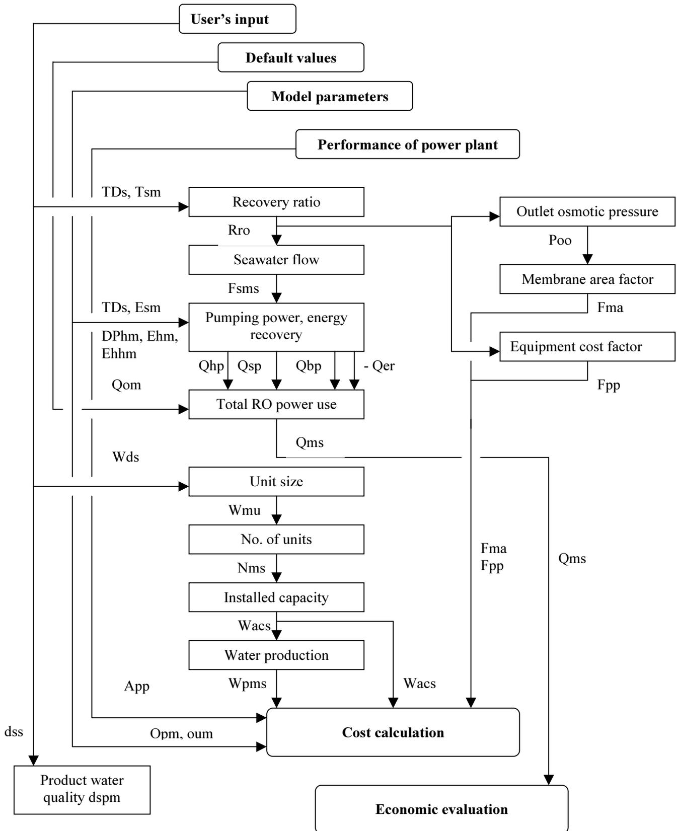
Fig 22. RO plant performance calculation.
