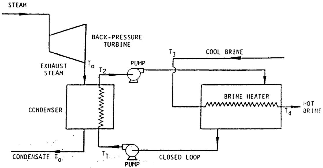
Fig. 9. Pressurised water isolation loop between backpressure condenser and MSF plant (just one MSF brine heater is shown for clarity).
