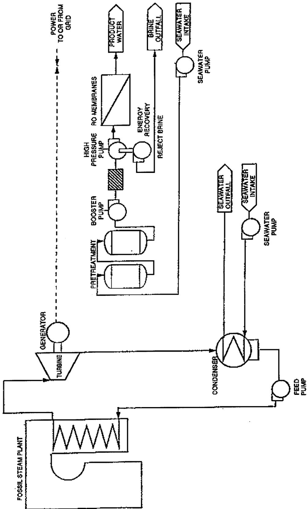
FIG. A-10. Fossil steam boiler with stand-alone RO system.
