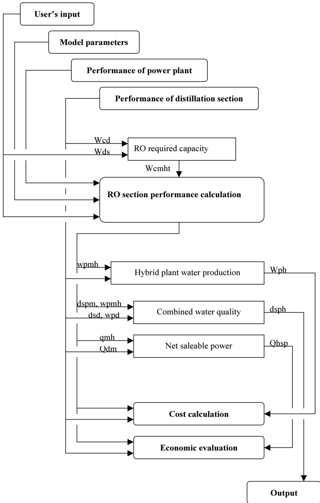
Fig 29. Hybrid plant performance calculation.
