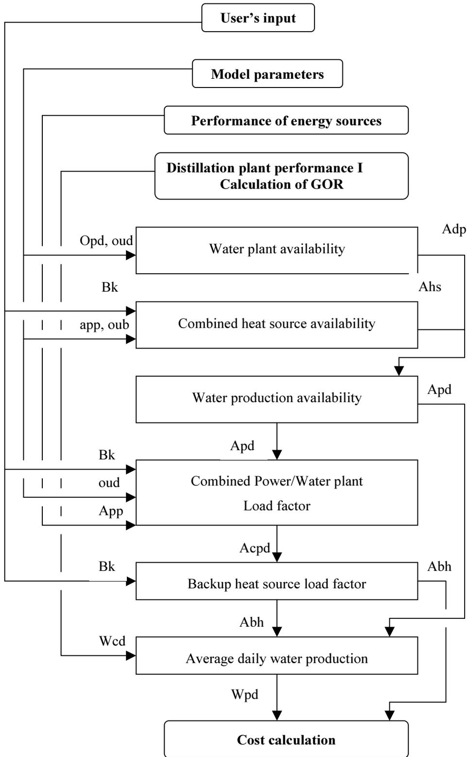
Fig 19. Distillation plant performance II – Calculation of water production.
