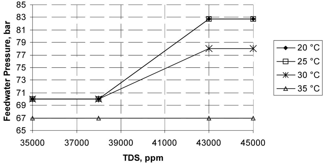
Fig 27. Feedwater pressure of hollow fibre membranes.
