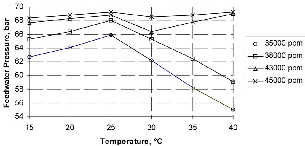
Fig 24. Feedwater pressure of spiral wound membranes.
