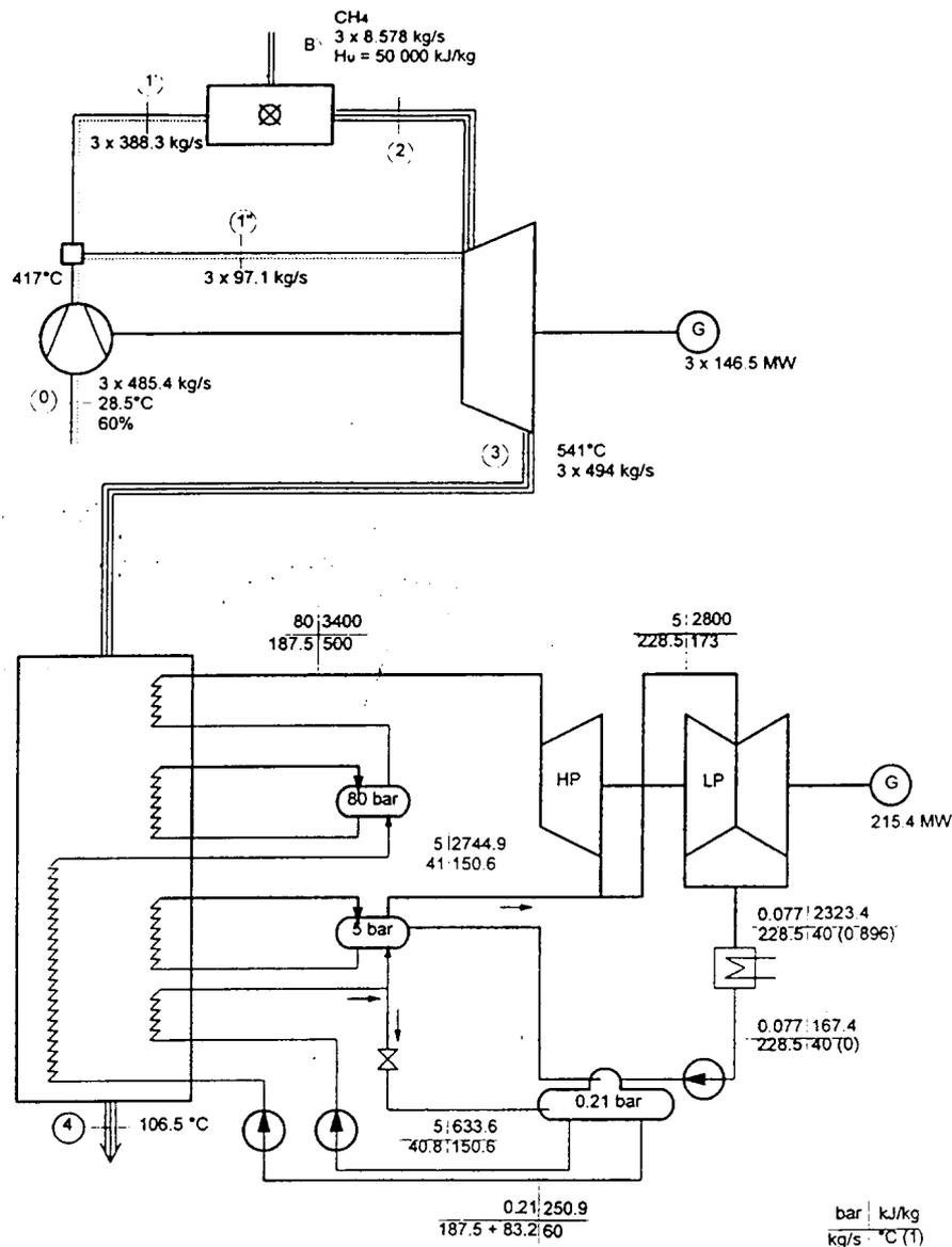
Fig. 5. Schematic flow diagram of the reference combined cycle.
