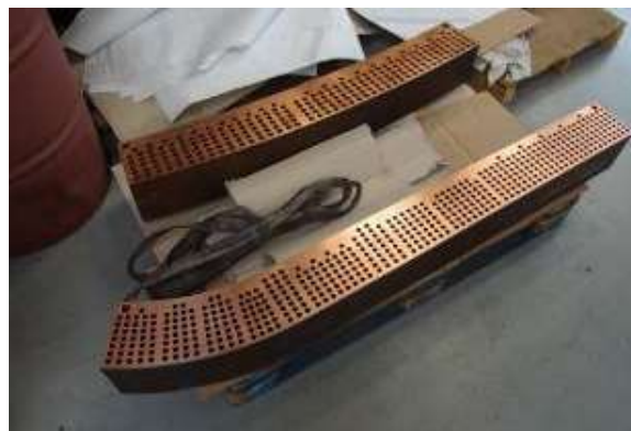
FIG. 10. Heater segments with drilled holes.
