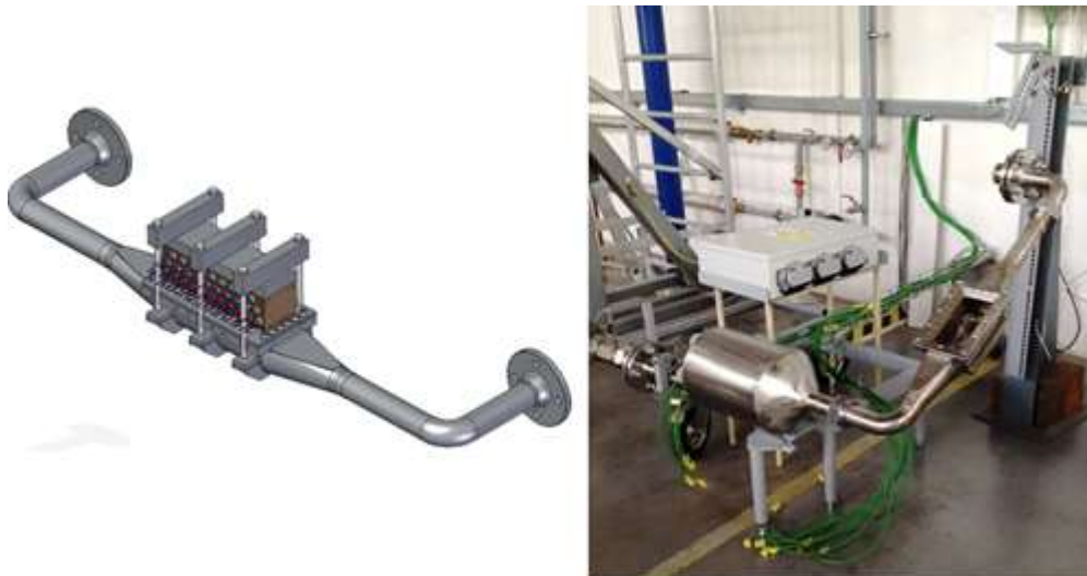
FIG. 2. Scheme of heating section and photo of heating section of BESTH2 facility [7].
