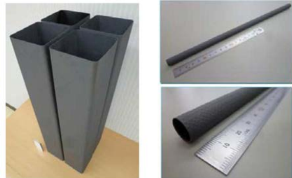
FIG. 5. Trial of Channel Box and Cladding Tube [9].
