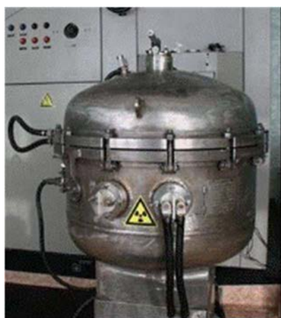
FIG. 2. Erosion Test Vessel at NNC [6].
