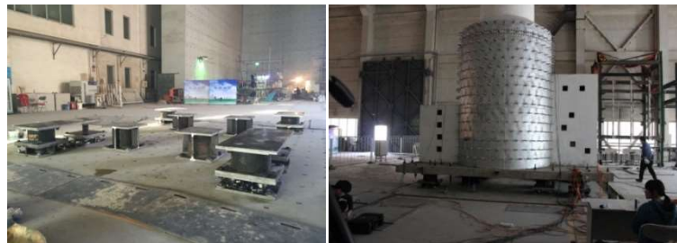
FIG. 3. Reduced-scale shaking table test.
