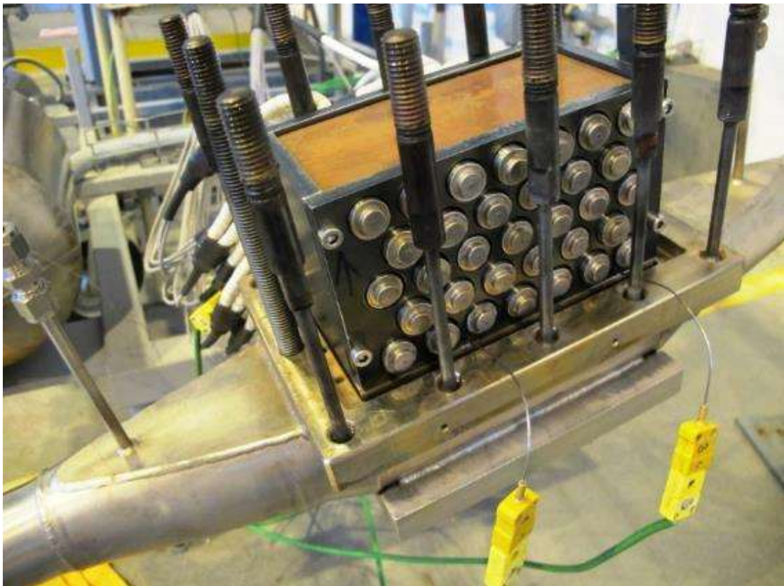
FIG. 4. Test sample with heating patrons and thermocouple position.
