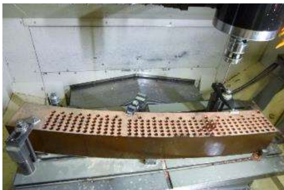
FIG. 10. Heater segments with drilled holes.
