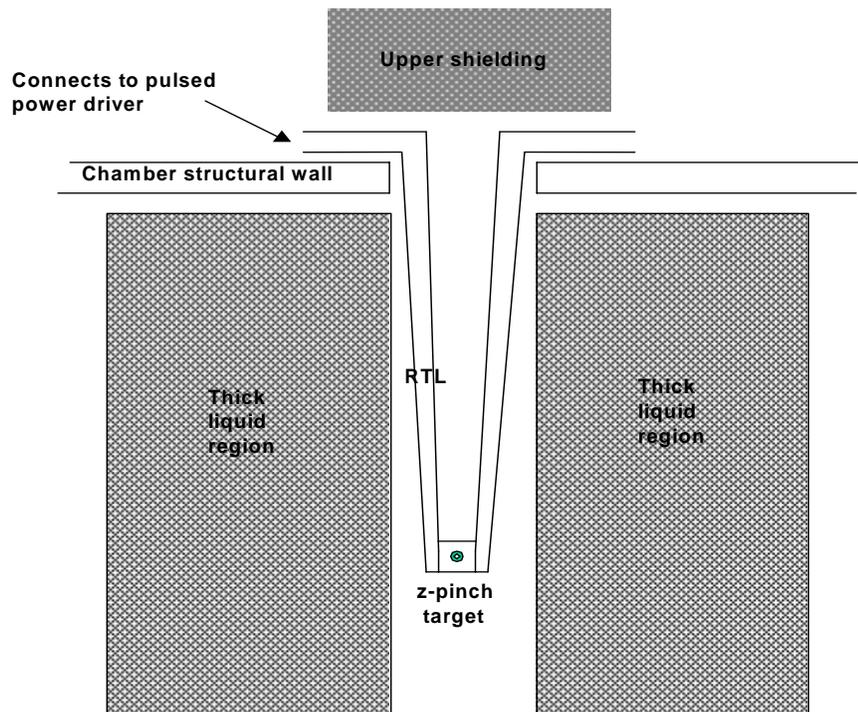
FIG. 2. The RTL (Recyclable Transmission Line) concept.
