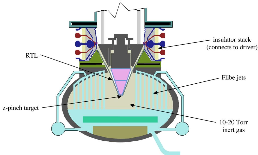
FIG. 6. Z-Pinch IFE chamber concept used in the ZP3 study [6,9].
