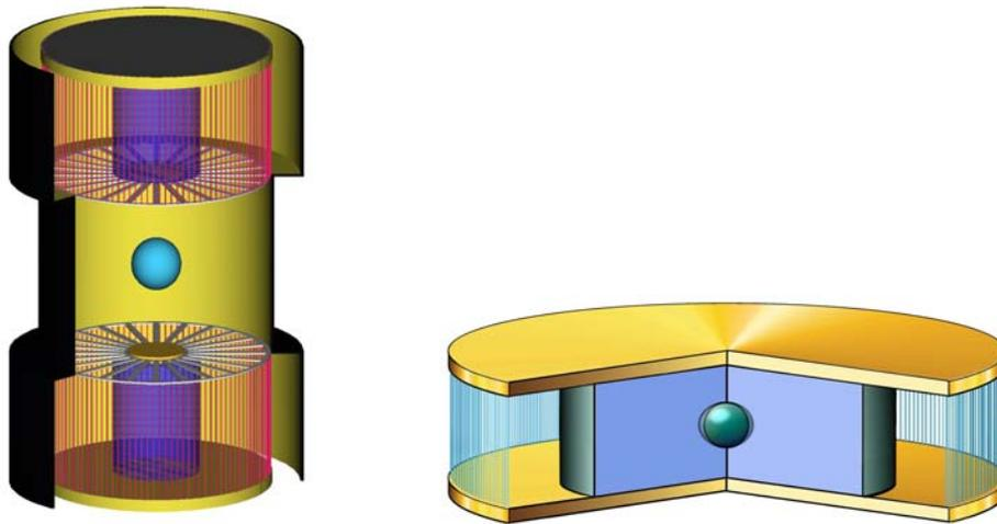
FIG. 5. Z-pinch fusion targets. The double-pinched target [32] is shown on the left, and the dynamic hohlraum target [33] is shown on the right.
