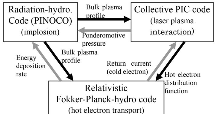
FIG.2 Data flow in FI<sup>3</sup> system. Black arrows are already executable data flows, and gray arrows are next plan to be considered.
