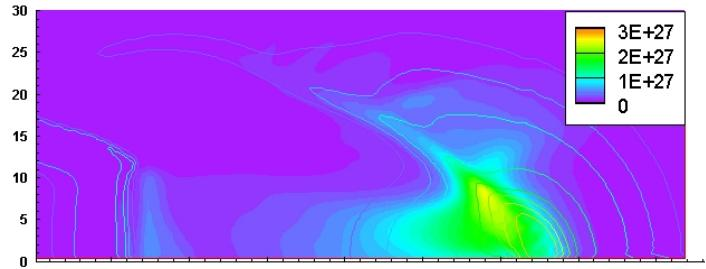
FIG.5. Contours of heating rate by fast electrons (color) and core density (line).
