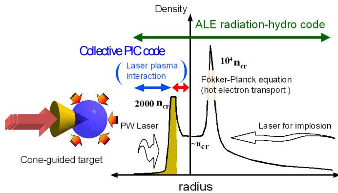
FIG.1. Fast Ignition Integrated Interconnecting code (FI<sup>3</sup>)
