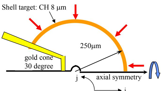
FIG.3. Initial condition of target
