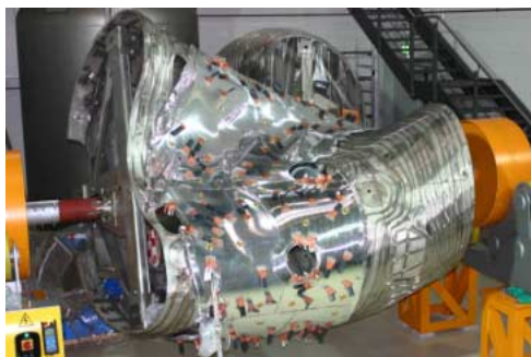
Fig. 5 Thermal insulation mounted onto one vessel half-module sector.
