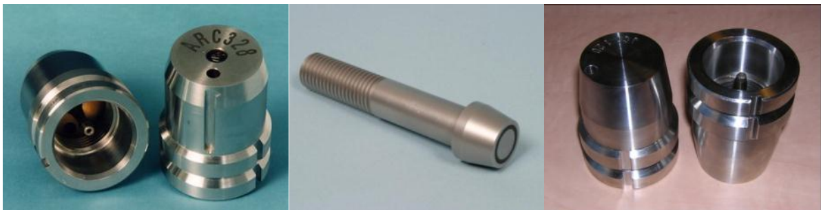
IAEA ultrasonic underwater seals (left to right): ARC (bolt head), USB (bolt + head), and JCSS (bolt head)
