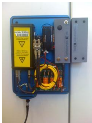
IAEA prototype door monitor (EOSS seal is used for events recording and communication)
