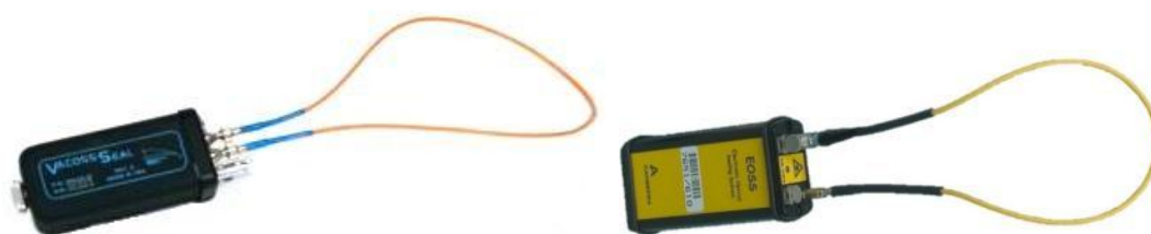
Current IAEA loop seals: VACOSS (left) and EOSS (right)
