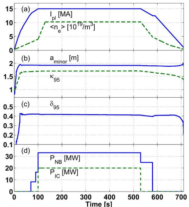
FIG. 2. ITER 15MA H-mode operation scenario. (a) The total plasma current, average electron density, (b) minor radius, plasma elongation, (c) plasma triangularity and (d) auxiliary H&CD powers are shown. Reprinted from Figure 2 of [5].
