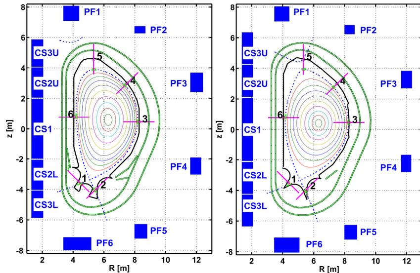
FIG. 3. Electromagnetic definitions of ITER for simulating the 15MA H-mode (left, [7], Reprinted from Figure 3 of [5]) and 12MA hybrid mode (right, [11]) scenarios. The PF coils (blue closed squares), vacuum vessel shells (green open squares), limiters (thick black lines), separatrix (blue dotted lines), six gap measurements between the plasma boundary and wall (violet lines with numbers) are shown.
