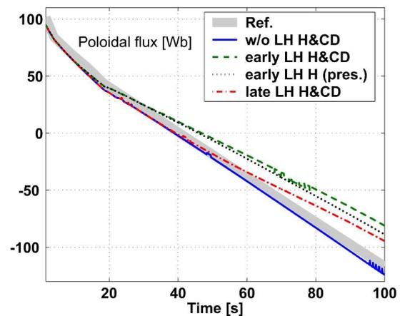
FIG. 6. Time traces of poloidal fluxes. Four cases, without LH H&CD, early LH H&CD, early LH H (heating profiles are obtained from early LH H&CD case, and then prescribed) and late LH H&CD are compared. Reprinted from Figure 5 of [6].
