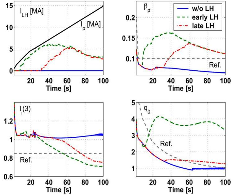
FIG. 5. Time traces of LH driven currents, poloidal plasma betas, internal inductances and central safety factor values. Three cases, without/early/late LH, are compared. Reprinted from the Figure 2 of [6].
