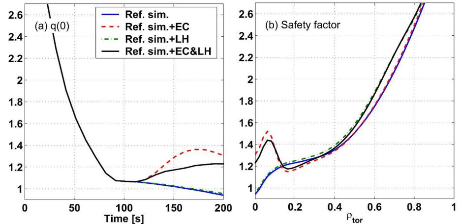
FIG. 8. (a) Time traces of central safety factors and (b) safety factor profiles at  $t=200$ s. Four cases, standard simulation, with additional 20MW of EC, with additional 20MW of LH and with both additional 20MW of EC and 20LW of LH. Repretined from figure 16 of [5]
