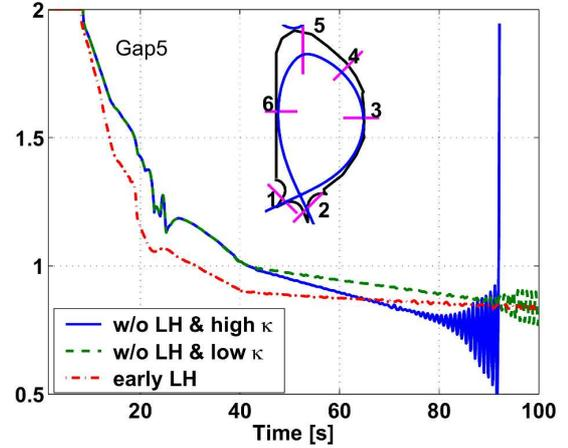
FIG. 7. Time traces of Gap 5 measured from the top of the vacuum vessel (see the nested small figure). Reprinted from figure 8 of [6].
