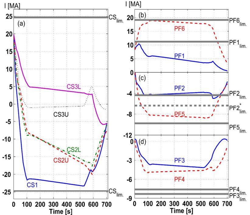
FIG. 4. Time traces of PF coil currents. The coil current limits are shown as thick grey lines. The PF2 coil current violated its limit ( $PF2_{lim.}$ ) around the end of the flat-top phase. However, in the recent ITER design review [13], this coil current limit has been increased in absolute value ( $PF2^*_{lim.}$ ). Reprinted from Figure 5 of [5].
