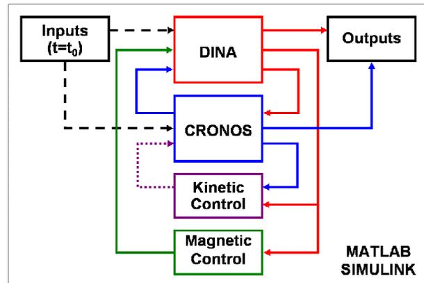
FIG. 1. Code coupling scheme used for the combined DINA-CH and CRONOS tokamak discharge simulator. Controlling the kinetic profiles is work in progress (dotted line). Reprinted from Figure 1 of [5].
