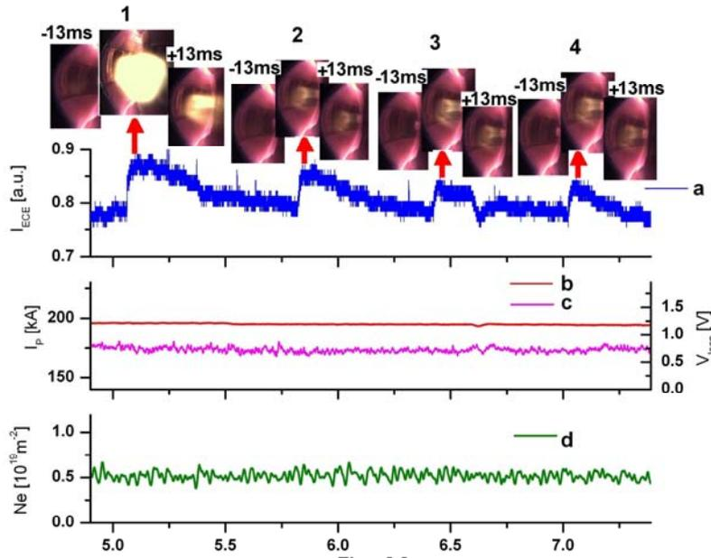
Fig.6. Top, pictures of CMOS camare clear show the FPASs. Four continuous FPAS events have occurred in about 3s. Bottom, the waveforms of other signals. a, the ECE intensity, b, the plasma current, c, loop
