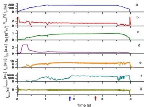
Fig.3. The waveforms of the discharge with synchrotron spot. a, the plasma current, b, loop voltage, c, the line average electron density, d, the electron temperature, e, the intensity of hard x-ray, f, the intensity of neutron, g, the Mirnov signal. The synchrotron spot observed with CMOS camera appeared from 1.8s. The picture in Fig. 2 was taken at 2.7s.
