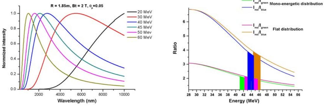
Fig.5. Left, The spectra of the synchrotron radiation. Right, The relation between the runaway energy and the ratios of the three color pixels. The shading bars are corresponded to the experimental data.
