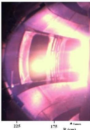
Fig.2. Typical synchrotron image obtained with the camera in a circular-configuration discharge
