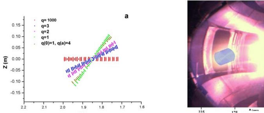
Fig.4. Numerical simulated shape of the synchrotron spot (poloidal projection) from 40MeV runaway beam with radius = 0.14 m in EAST. Left, The radiation pattern with different  $q$  and fixed pitch angle ( $\theta_p = 0$ ).  $q = 1000$  means there is no helical structure for the magnetic field. Right, the radiation pattern (blue curves) with  $\theta_p = 0.05$ , which is overlapped into the same image of figure 2. A parabolic-like  $q$  profile is assumed ( $q(0) = 2.8$ ,  $q(a) = 6.5$ ).
