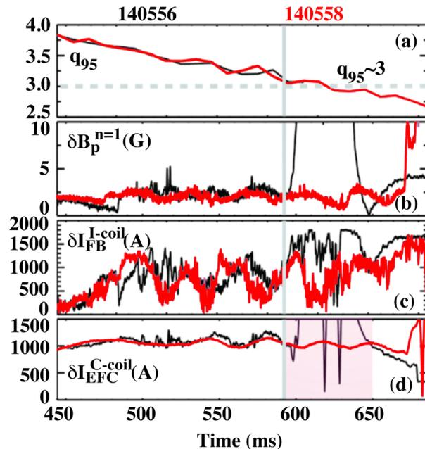
FIG. 2. Simultaneous operation of feedback-controlled EFC and DF on the unstable RWM at  $q_{95} \sim 3$  with optimized gains (in red) and with lower gains (in black). Shown are the time traces of (a) edge safety factor  $q_{95}$ , (b)  $n=1$  magnetic perturbations on poloidal field probes, (c) internal feedback coil currents, and (d) external EFC coil currents.
