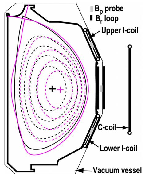
FIG. 1. Poloidal cross-section of low- $\beta$  (in black) and high- $\beta$  (in magenta) plasmas used for feedback-controlled EFC and RWM stabilization study in DIII-D. Shown are the upper single null (close to double-null) plasmas with magnetic sensors (poloidal field probes and radial field loops) and coils [internal (I-coils) and external (C-coils) to the vacuum vessel].
