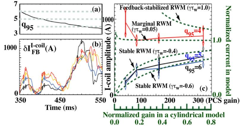
FIG. 3. Stable, marginal and feedback-stabilized RWMs. Left: time traces of (a) edge safety factor  $q_{95}$ , and (b) internal feedback coil (“I-coil”) currents at various gains ( $G_p=40, 80, 160$  and  $320$  from the bottom respectively). In (c), the gain dependency of the I-coil currents varies subject to the RWM regimes, which is consistent with the predictions (dashed curves) of a cylindrical model [11].
