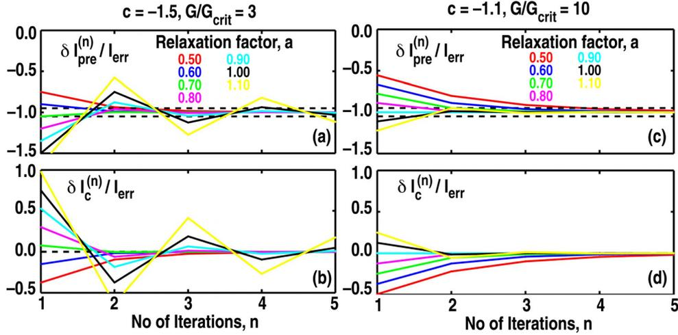
FIG. 4. Pre-programmed EFC coil currents  $\delta I_{pre}$  and feedback coil currents  $\delta I_c$  normalized to error field  $I_{err}$  vs no. of iterations at various relaxation factors in model. In (a) and (b), a low gain ( $G/G_{crit}=3$ ) is considered, while in (c) and (d), a high gain ( $G/G_{crit}=10$ ) is under consideration. The dashed lines in (a) and (c) are the target area within  $\pm 5\%$  uncertainty, while those with  $\delta I_c = 0$  in (b) and (d) are the ideal targets.
