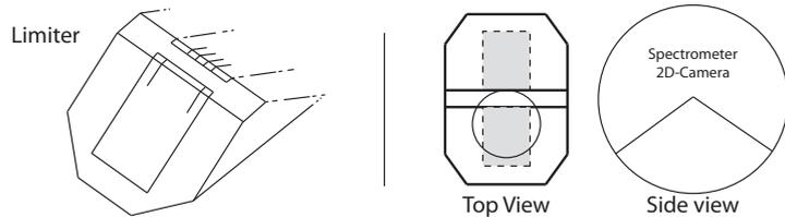
**Figure 1:** (Left) Limiter setup (Right) Diagnostic views (Circle = pyrometer). Gray areas indicate tiles ( $3.5cm \times 5.5cm \times 0.2cm$ ).
