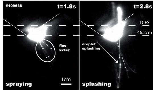
**Figure 6:** Melt layer ejection, spraying(left) and splashing(right), LCFS is indicated [11].
