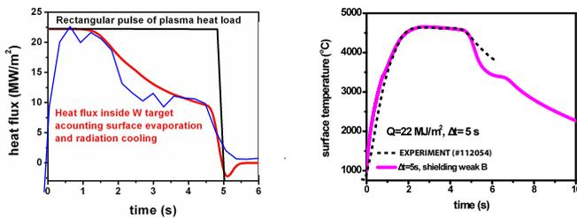
**Figure 9:** Heat flux and temperature Data vs. MEMOS [24, 25]
