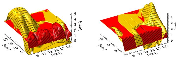
**Figure 4:** (Left - 2L), (Right - 2H) Profiles before (red) and after exposure (golden)
