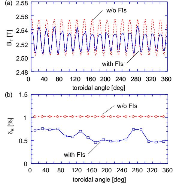
FIG. 2. (a) The  $B_T$  along the toroidal angle at the separatrix on the outer midplane ( $R=4.28\text{m}$ ,  $Z=0.2\text{m}$ ) for the cases before and after the installation of FIs in JT-60U. (b) The TF ripple at each section between 2 TF coils.
