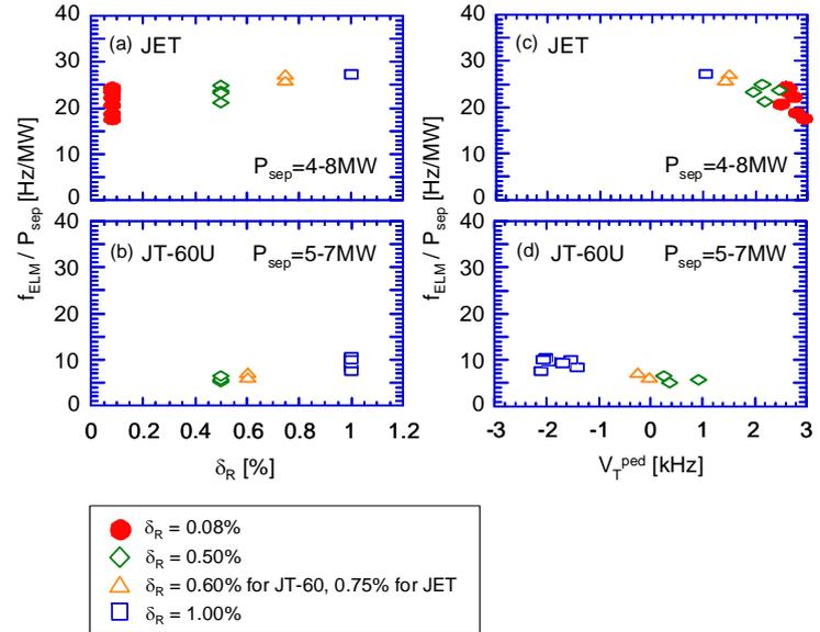
FIG. 10. ELM frequency normalized to the power crossing the separatrix observed in JET and JT-60U as a function of  $\delta_R$  and  $V_T^{ped}$ .
