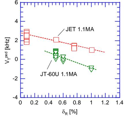
FIG. 4. The toroidal rotation velocity at the H-mode pedestal shoulder  $V_T^{\text{ped}}$  as a function of  $\delta_R$ . Squares and inverse triangles indicate the data taken from the similarity experiment at 1.1MA in JET and JT-60U, respectively. The TF ripple scan conducted using the JET standard configuration at 2.6MA is also plotted as triangles for reference.
