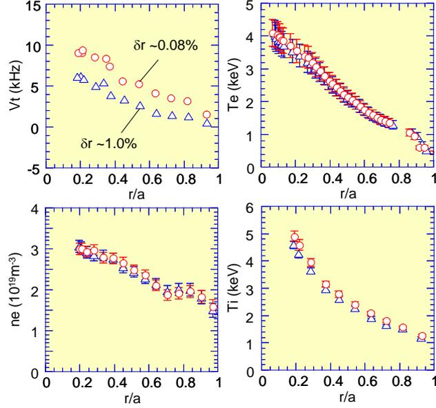
FIG. 7. Spatial profiles of  $V_t$ ,  $n_e$ ,  $T_e$  and  $T_i$  for the TF ripple scan experiment in JET. Circles and triangles denote the TF ripple amplitude of 0.08% and 1.0%, respectively.
