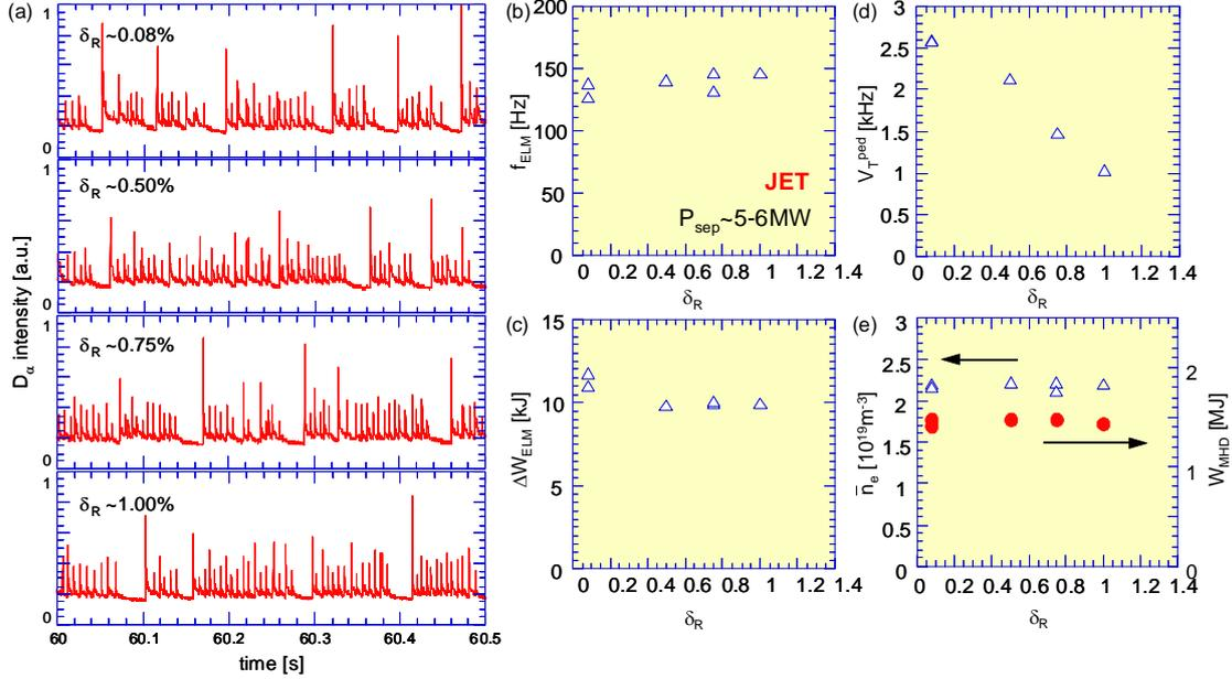
FIG. 9. (a)  $D_\alpha$  emission intensity at the outer divertor for the variation of TF ripple in JET. Dependence of TF ripple on (b) ELM frequency, (c) ELM energy loss, (d) edge toroidal rotation frequency, (e) line-averaged electron density, and total stored energy.
