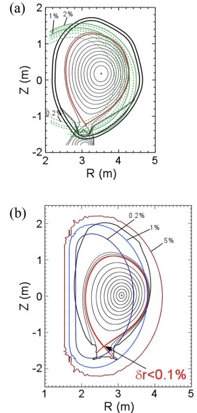
FIG. 1. Plasma cross sections for the similarity experiments together with TF ripple amplitude  $\delta_R$  in (a) JT-60U and (b) JET. Here,  $\delta_R$  is defined as  $(B_{TMax} - B_{TMin}) / (B_{TMax} + B_{TMin})$ . The number of TF coils is 18 in JT-60U and 32 in JET.
