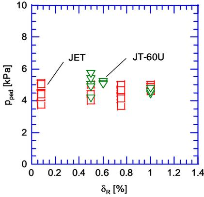
FIG. 6. Dependence of pedestal pressure on  $\delta_R$ . Squares and inverse triangles denote the similarity experiment at 1.1MA in JET and JT-60U, respectively.
