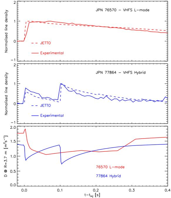
FIG.6. The post pellet line density evolution is well reproduced by JETTO simulations using a BgB diffusion coefficient (bottom) with an enhanced factor of 3-8 in the pellet deposition zone.
