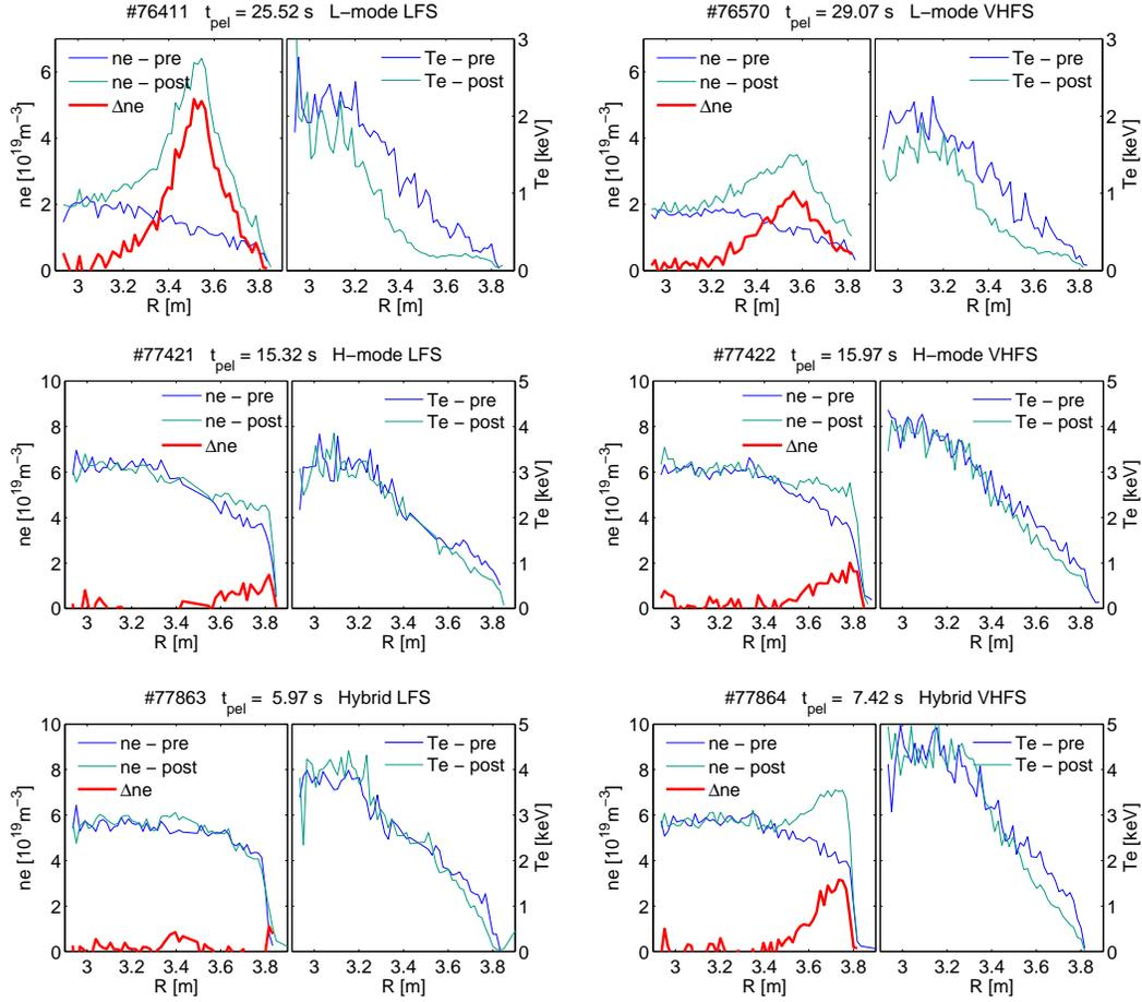
FIG. 3. Density and temperature profiles before and immediately after pellet injection as measured by the Thomson Scattering. Particle deposition ( $n_{post}-n_{pre}$ ) is also shown in the density box/ Top: L-mode (5 MW); Middle: H-mode(10 MW); Bottom: Hybrid (21
