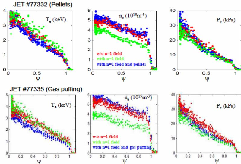
FIG. 9. Electron temperature, density and pressure profiles before and during ELM mitigation experiments with resonant magnetic perturbation ( $n=1$ ). The density pump-out is compensated by pellets (top row) or by gas fuelling (bottom row). (Liang)
