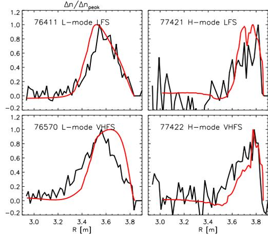
FIG. 4. Experimental particle deposition compared with simulations performed with HPI2 with zero  $\nabla B$  drift (red) Particles injected from VHFS show a moderate inward drift.
