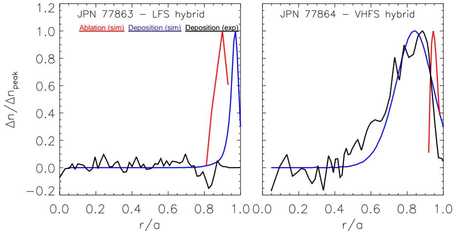
FIG.5. Simulations with HPI2 show a clear effect of  $\nabla B$  drift on pellets injected from the LFS (left) and VHFS (right) into high power (~21 MW) hybrid discharges. Particles injected from LFS are rapidly displaced outwards and leave the main plasma, while in the VHFS case they are shifted inwards producing a significant modification of the density profile.
