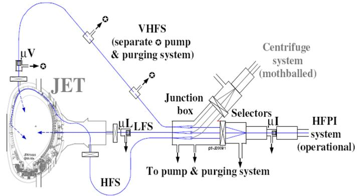
FIG. 1. Schematic of the pellet injection system.
