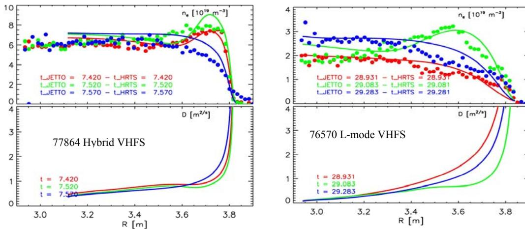
FIG. 7. Experimental density profiles compared with simulations. In the bottom boxes, the corresponding profiles of the particle diffusion coefficients are shown
