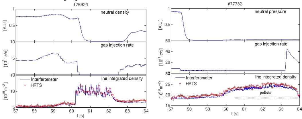
FIG. 8. Divertor neutral density, gas injection rate and central line average electron density during the injection of a 5 Hz pellet train in L (left) and H (right) mode.
