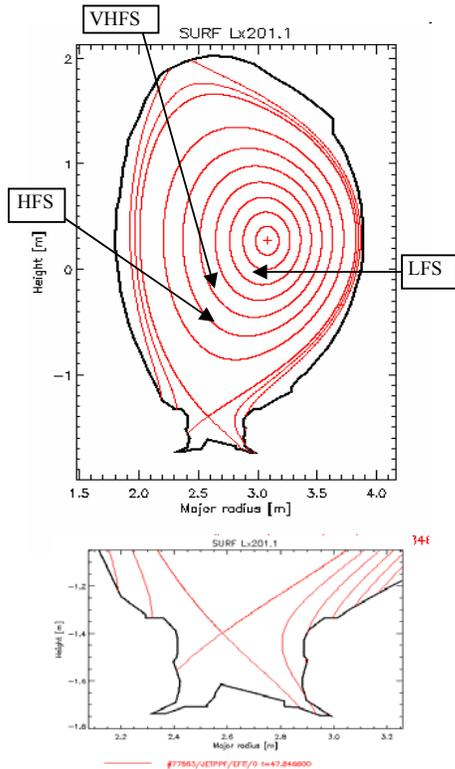
FIG. 2 .Top: JET plasma geometry and aims of pellet injection trajectories. Bottom: details of the Divertor field lines
