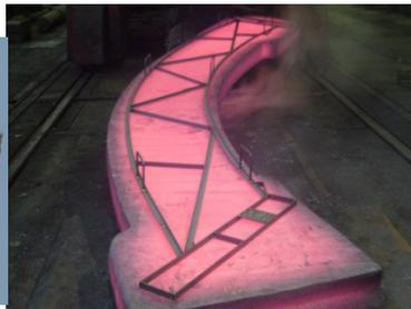
Radial plate mock-ups for TF coil produced by HIP (left) and forging (right) (EU)
