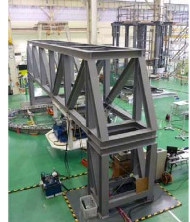
Tooling for 1/3 scale dummy winding (JA)
