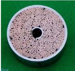
TF conductor (Nb<sub>3</sub>Sn)
