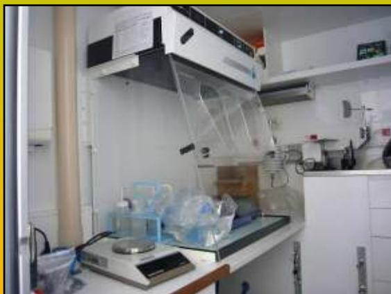
The Sample is decontaminated beforehand by precipitating hydroxides with ammonia in chlorydric milieu. After regrowing from purified strontium-90, yttrium-90 is extracted in organisical phase, then measured liquid scintillation.
