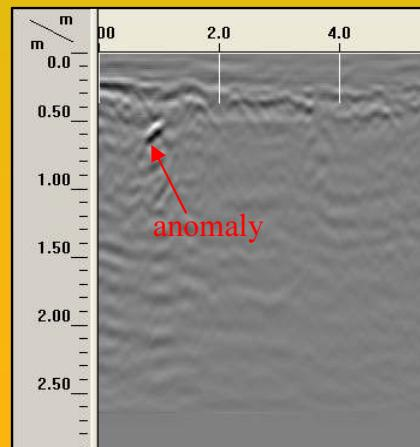
Confirm the position of drill holes by checking the absence of metallic parts or underground network near the drill holes.
