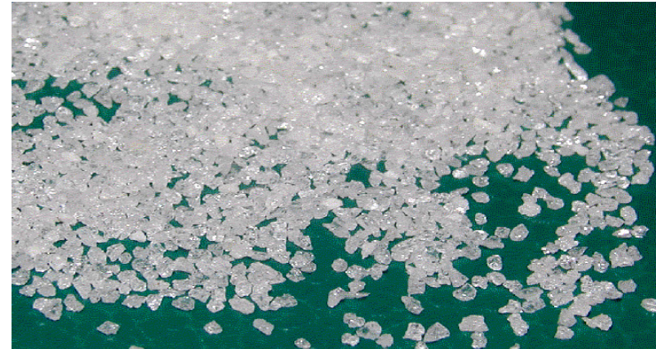
Metallographic specimen grain \text{Al}_2\text{O}_3 (granule size d=0.8-1.0\ \text{mm} , t\leq 800^\circ\text{C} )
