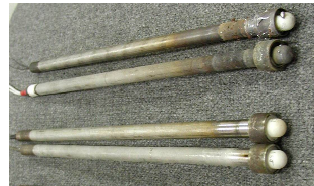
New generation of the sensors controlling thermodynamic activity of dissolved oxygen
