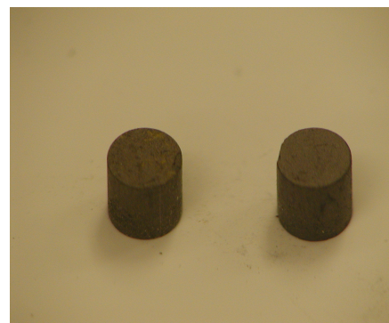
U_{0.805}Pu_{0.175}Am_{0.02}N nitride fuel pellets
