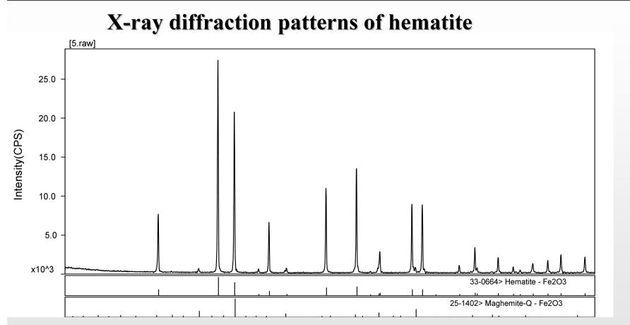
It can't be seen the diffraction peaks of crystals formed by uranium. It may be explained that the complex formed by U(VI) in neuter solution didn't form crystal lattice after adsorption to the surface of hematite with the function of electrostatic force.
