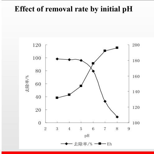
As the initial pH increased, the removal rate of U (VI) decreased, when pH was over 5, it decreased rapidly . At acid condition, uranium existed as  $UO_2^{2+}$  which was reduced by ZVI suitable, when near neutral and alkaline, it existed as other complexions, these complexions inhibited the reduction of uranium, oxidation-reduction potential increasing with pH increasing, illustrated that the decreased
