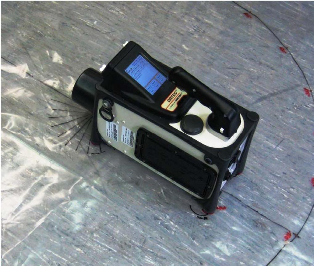
Electrically cooled HPGe with battery power supply and integrated software for analysis.
