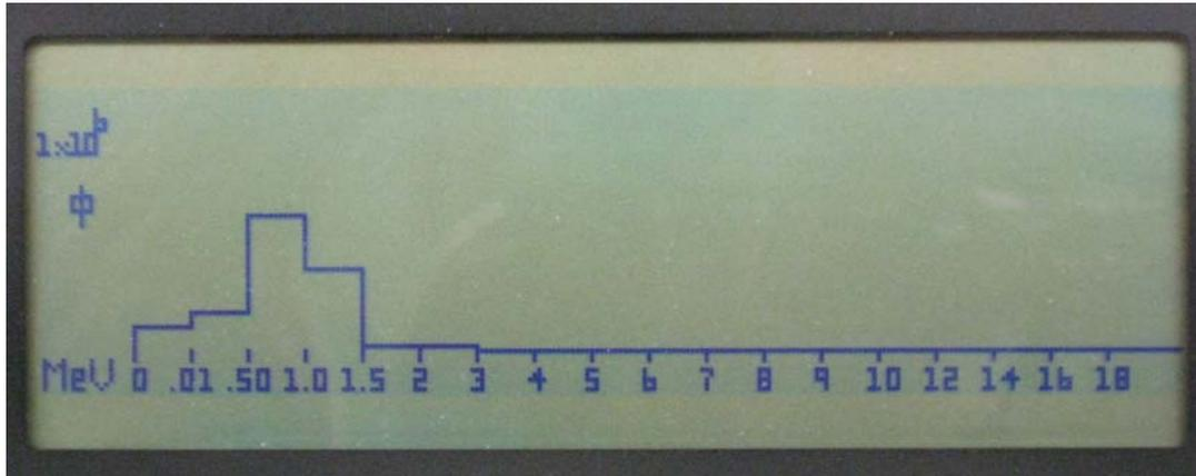
Display of the neutron spectrum (neutron fluence)
